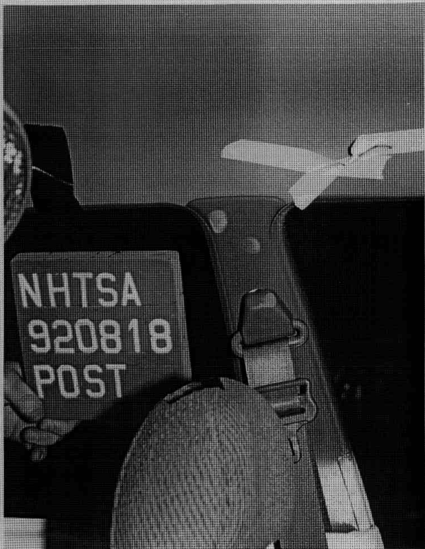
FIGURE A-41. POST-TEST DRIVER DUMMY HEAD CONTACT - VIEW 4
