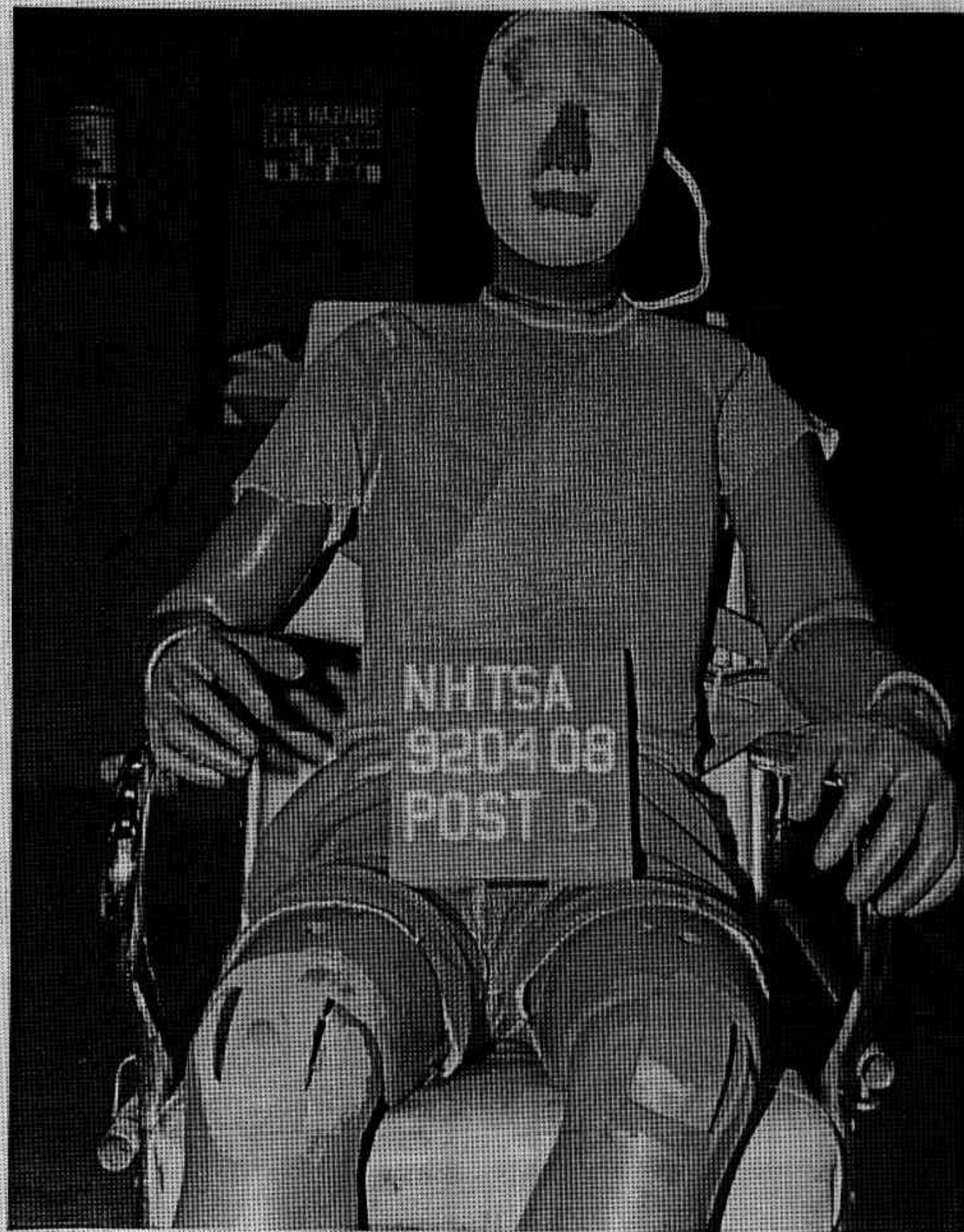
FIG. A-38. POST-TEST DRIVER DUMMY HEAD, CHEST, & KNEE CONTACT - VIEW 1
