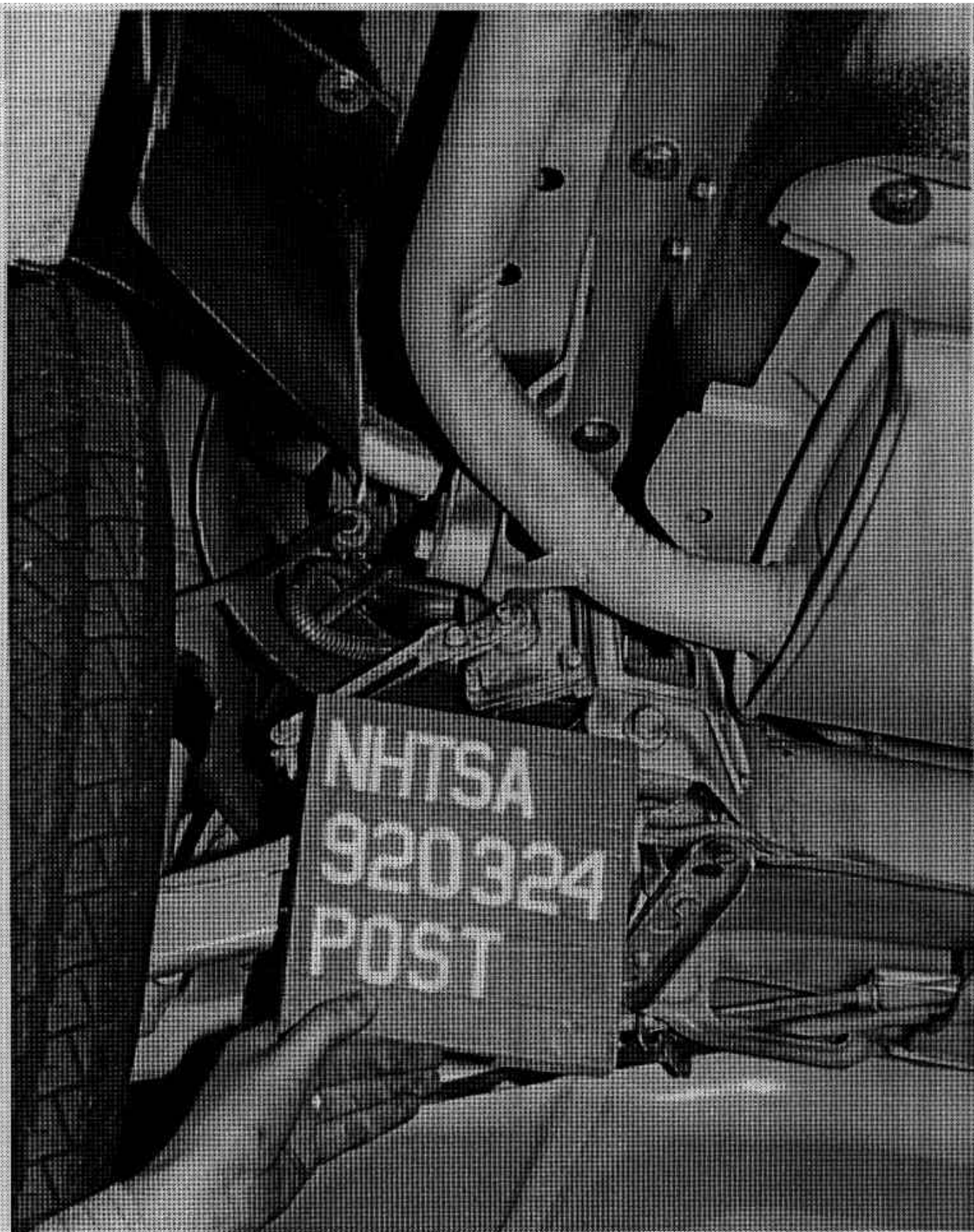
FIGURE A-20. POST-TEST FUEL FILLER NECK VIEW
