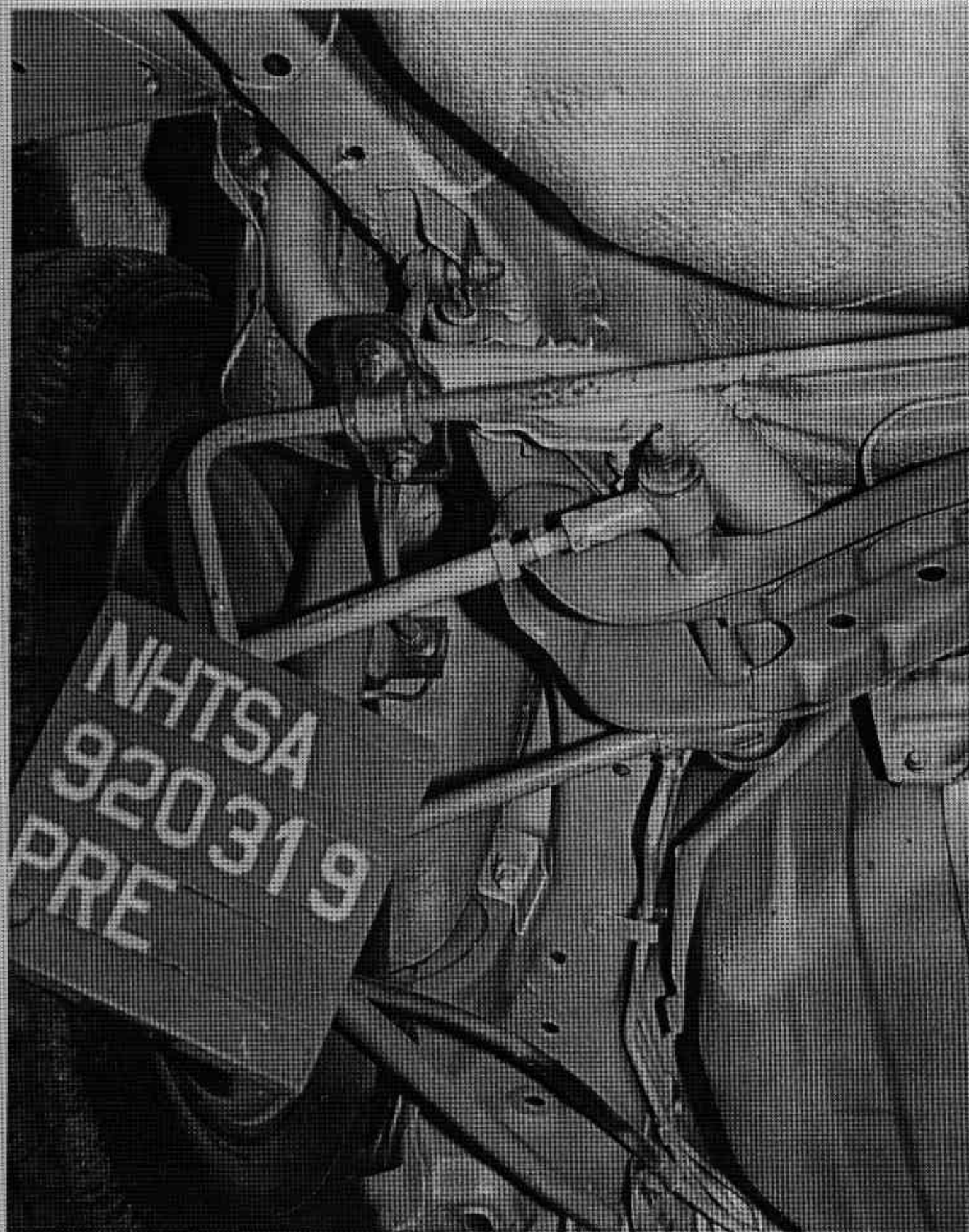
FIGURE A-18. PRE-TEST FUEL FILLER NECK VIEW
