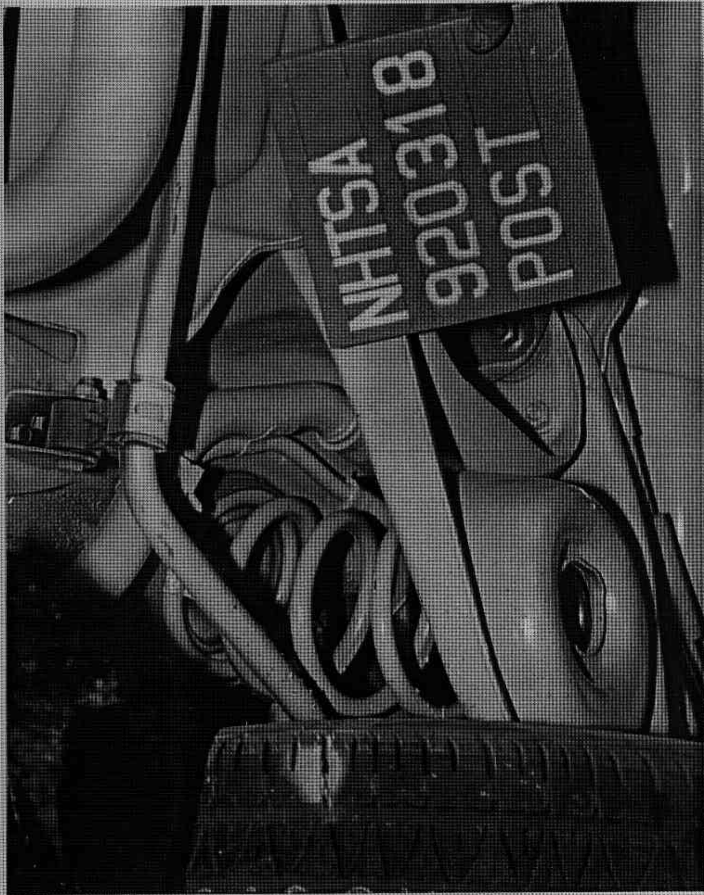
FIGURE A-20. POST-TEST FUEL FILLER NECK VIEW
