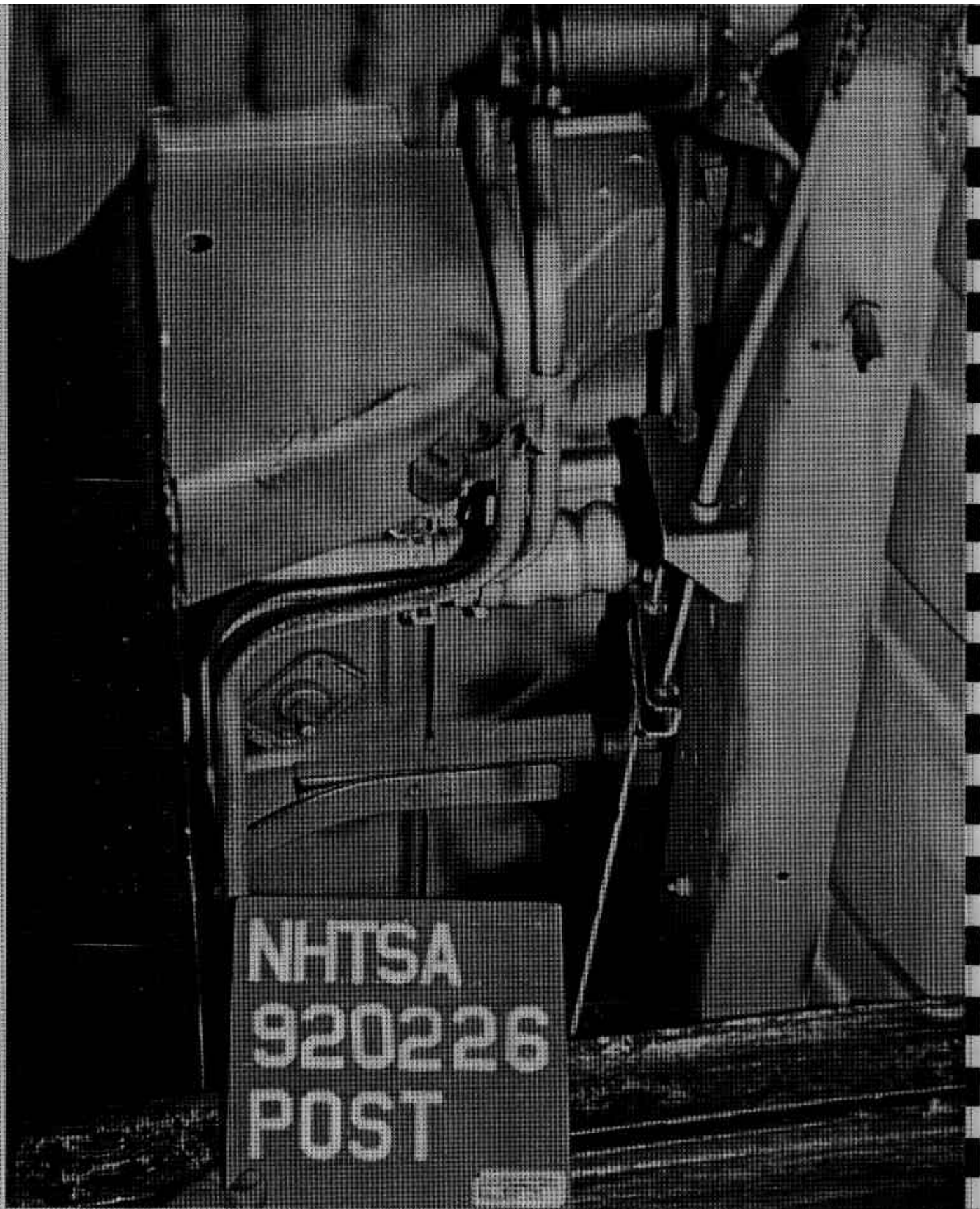
FIGURE A-20. POST-TEST FUEL FILLER NECK VIEW
