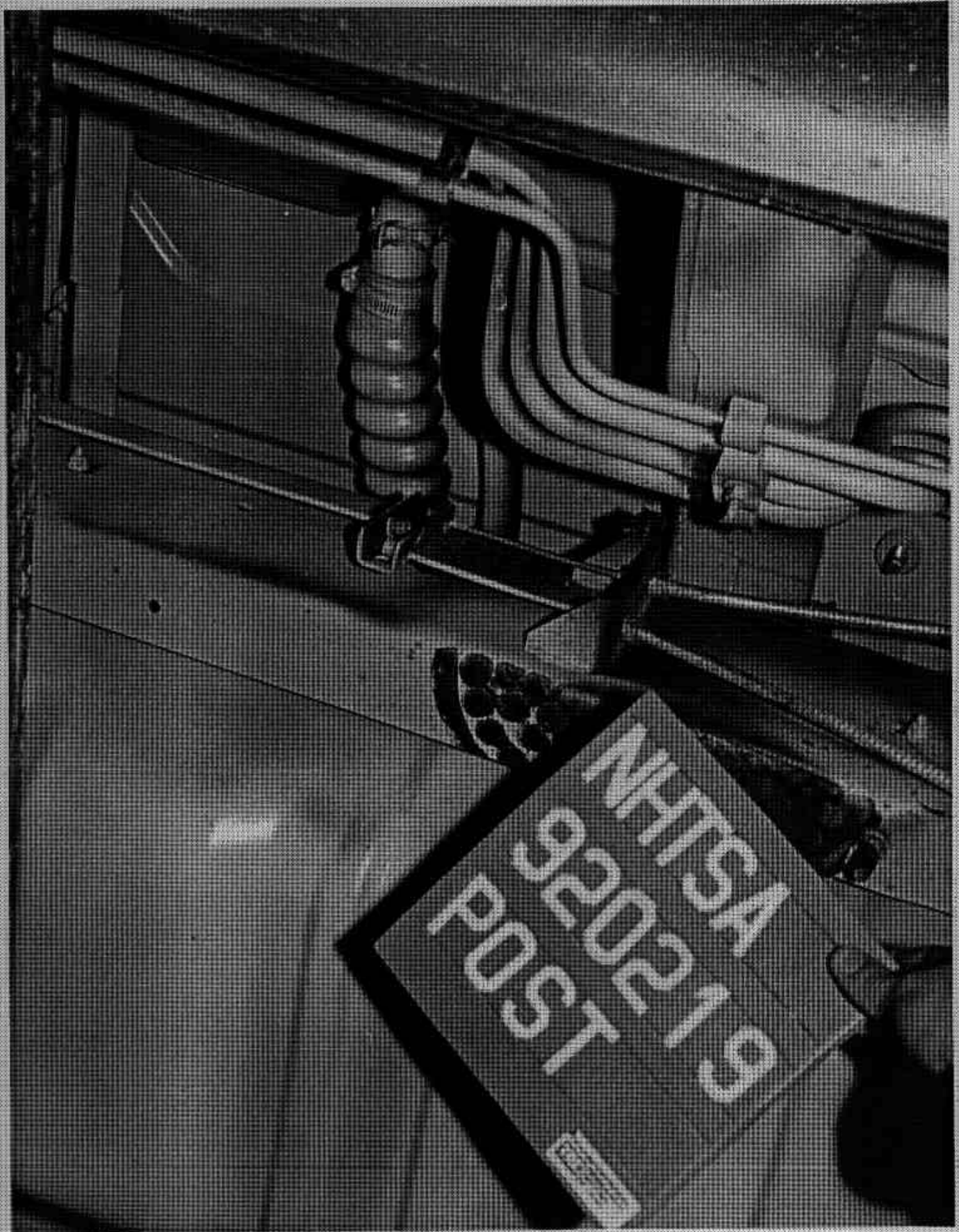
FIGURE A-20. POST-TEST FUEL FILLER NECK VIEW
