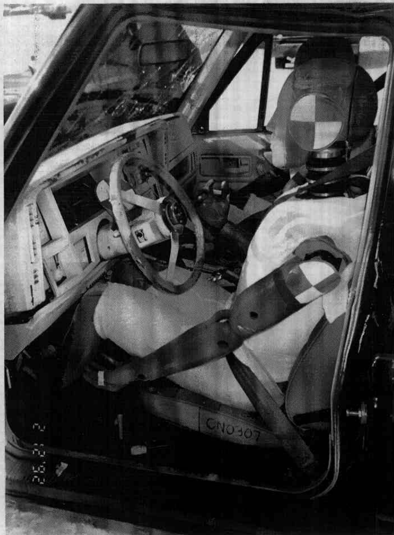
Figure A-30 POST-TEST DRIVER DUMMY AND INTERIOR VIEW
