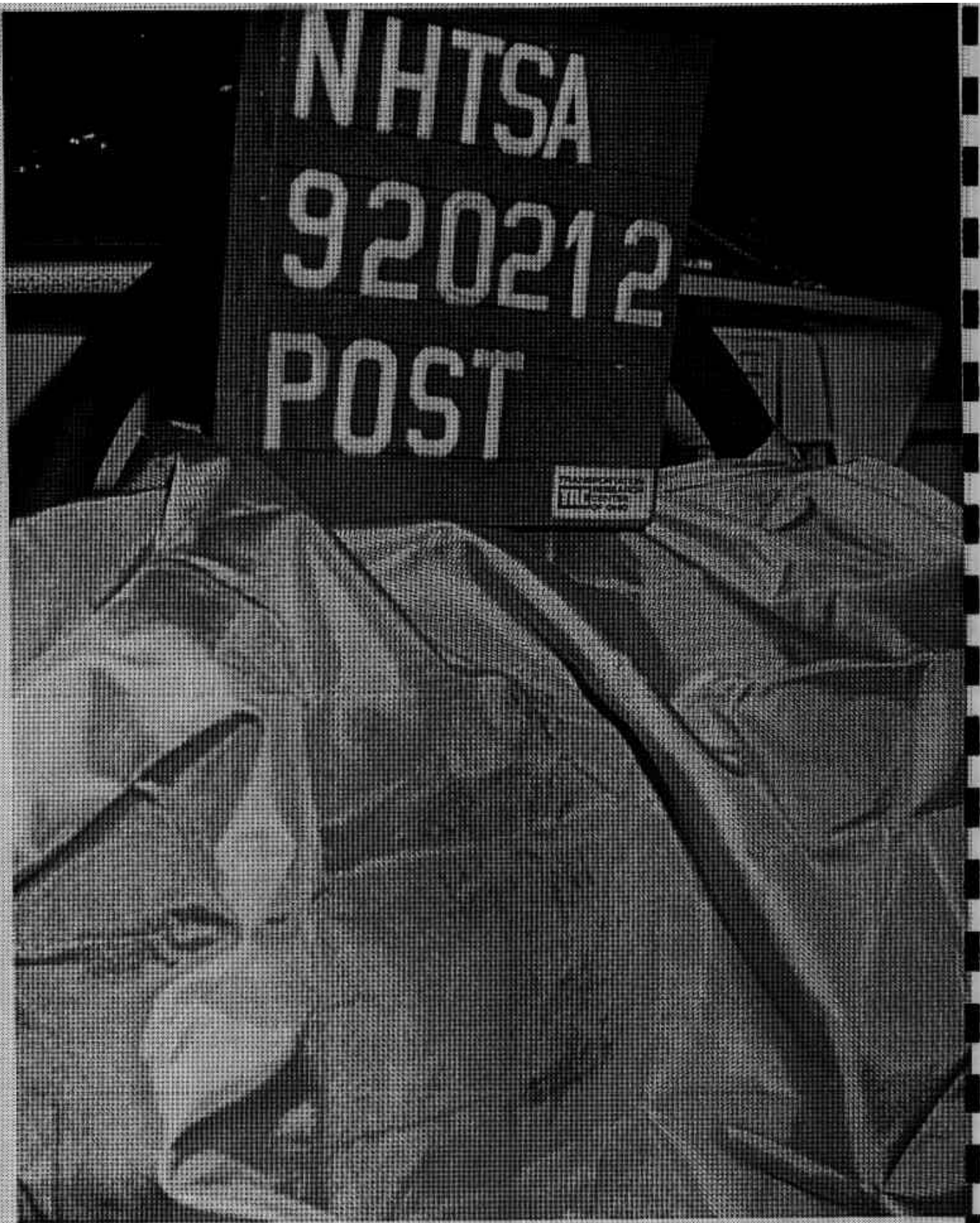
FIGURE A-38. POST-TEST DRIVER DUMMY HEAD CONTACT - VIEW 2
