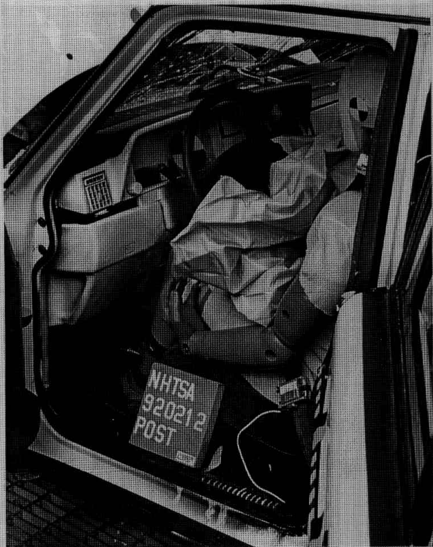
FIGURE A-32. POST-TEST DRIVER DUMMY & VEHICLE INTERIOR - VIEW 2
