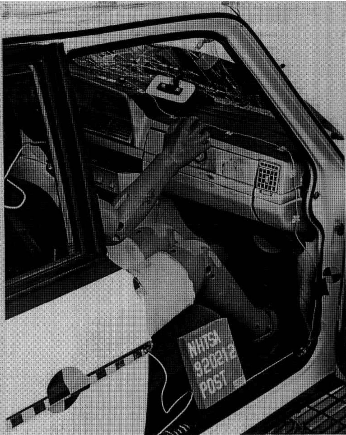
FIGURE A-36. POST-TEST PASSENGER DUMMY & VEHICLE INTERIOR - VIEW 2 A-37 920212
