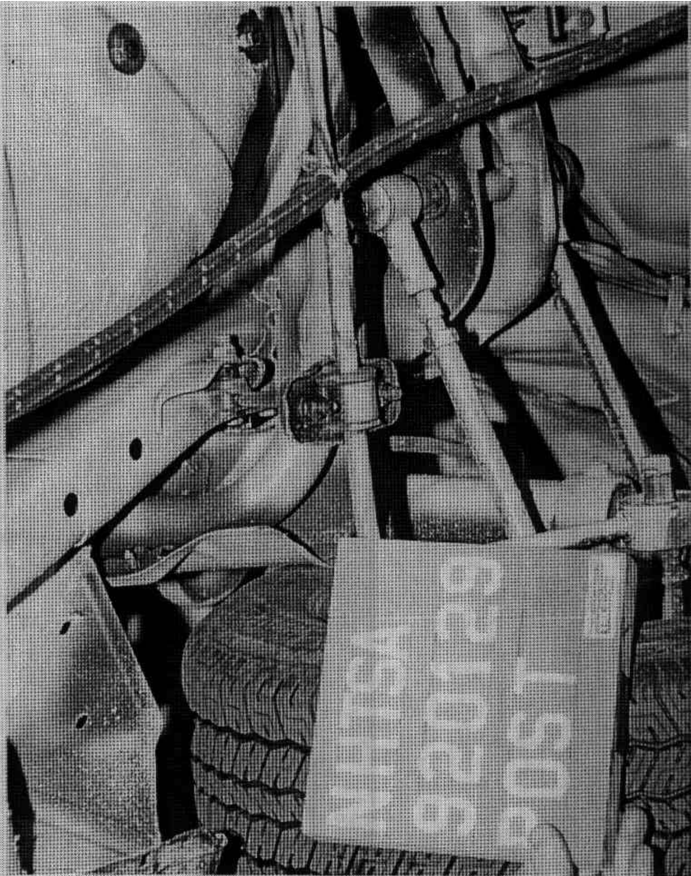
FIGURE A-20. POST-TEST FUEL FILLER NECK VIEW
