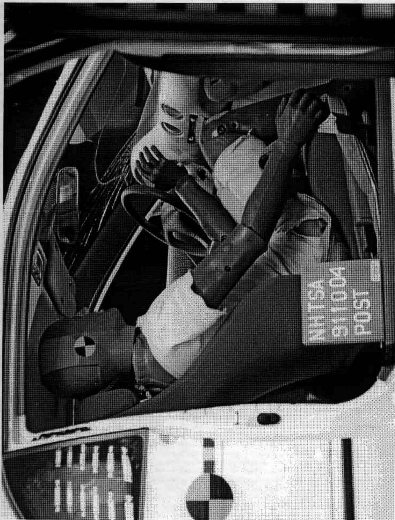
FIG. A-35 POST-TEST PASSENGER DUMMY & VEHICLE INTERIOR - 1
