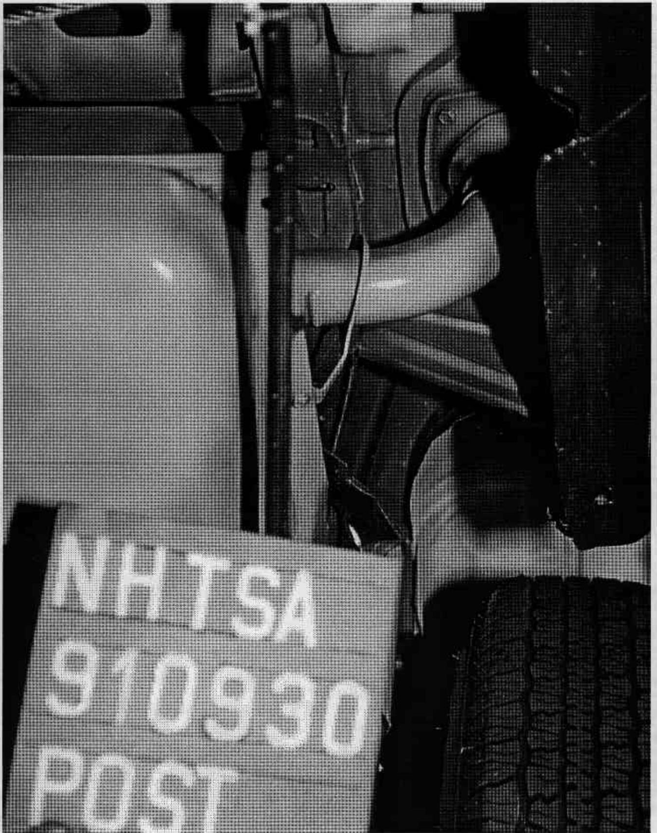
FIGURE A-20 POST-TEST FUEL FILLER NECK VIEW
