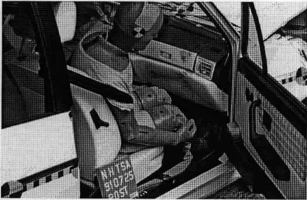
Fig A-37. POST-TEST PASSENGER DUMMY & VEHICLE INTERIOR VIEW 2
