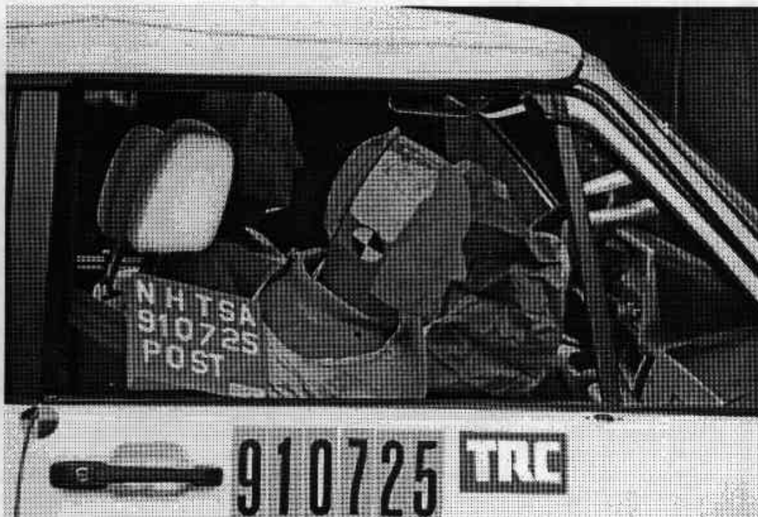
Fig A-29. POST-TEST PASSENGER DUMMY POSITION VIEW
