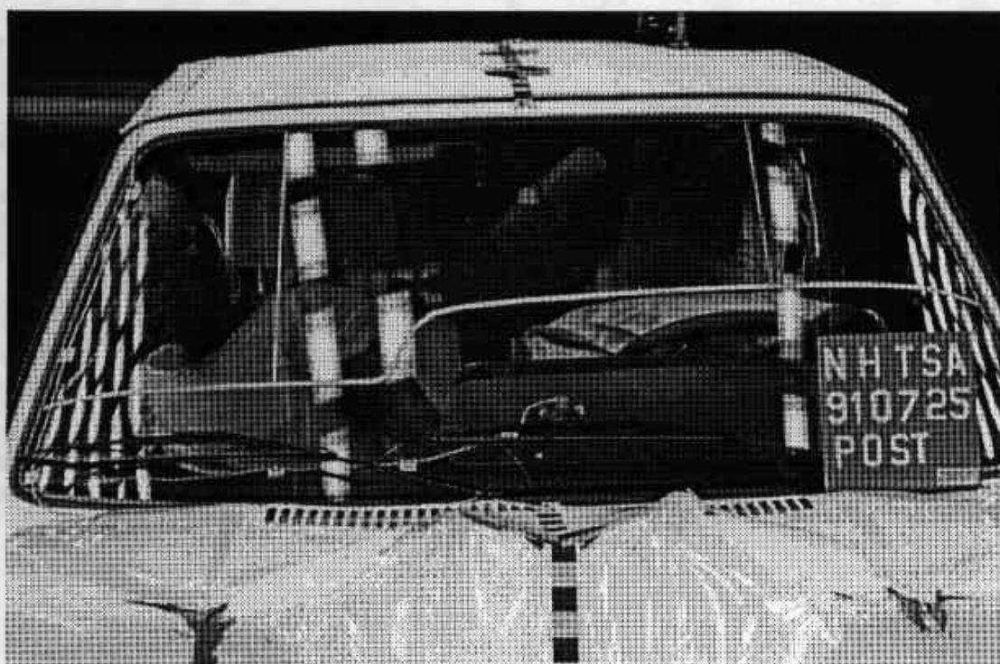
Figure A-14. POST-TEST WINDSHIELD VIEW
