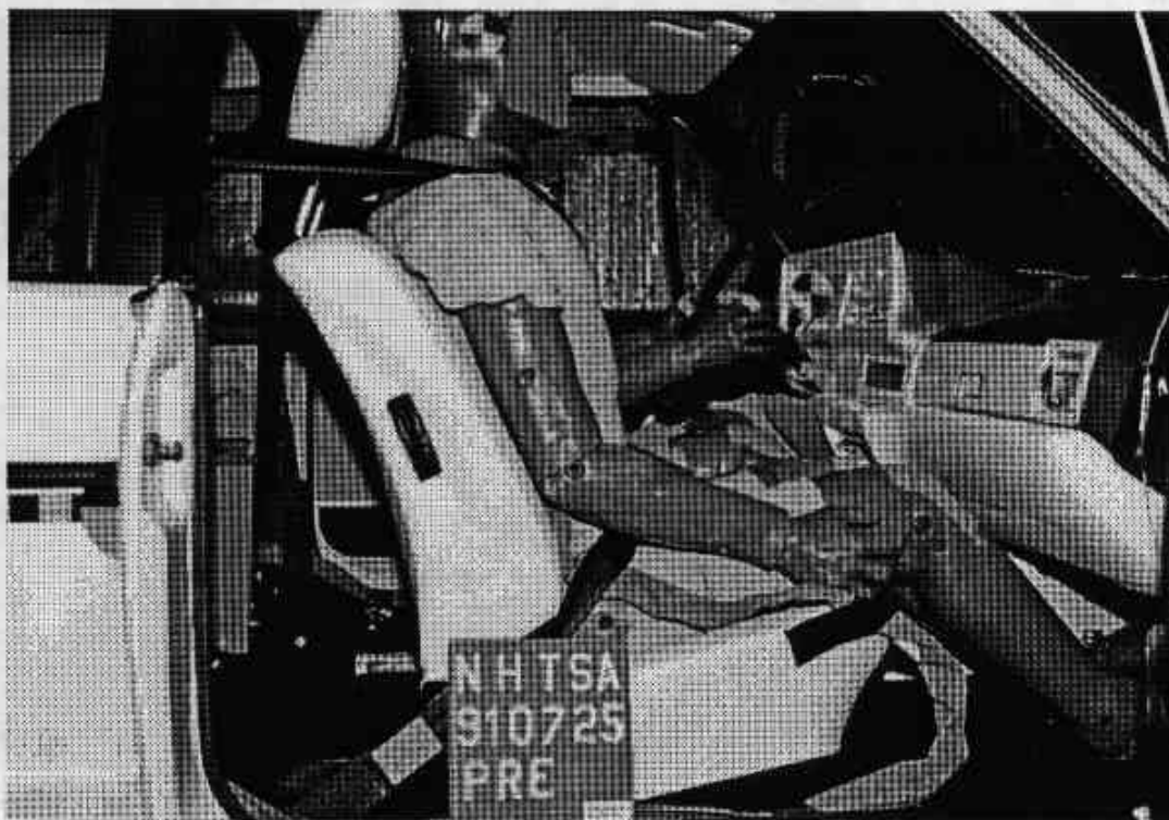
Fig A-34. PRE-TEST PASSENGER DUMMY & VEHICLE INTERIOR VIEW 1
