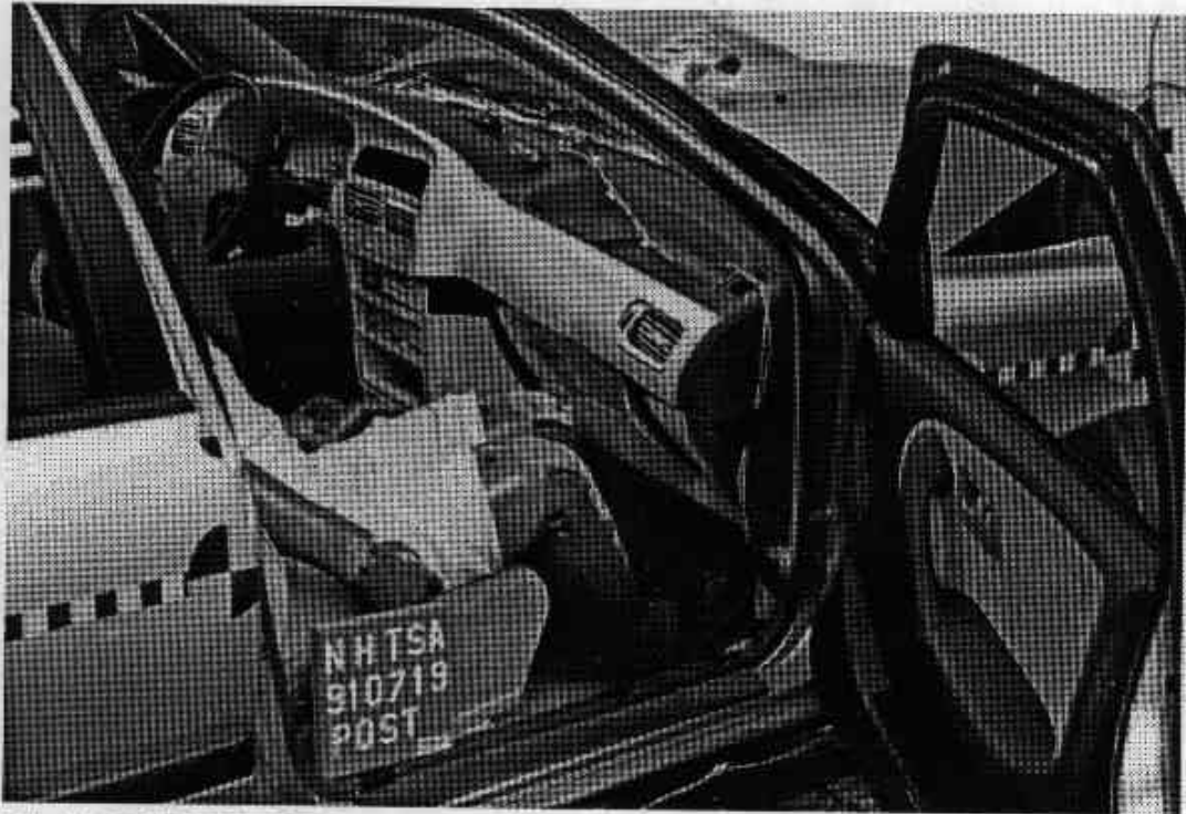
Fig A-33. POST-TEST PASSENGER DUMMY & VEHICLE INTERIOR VIEW 2
