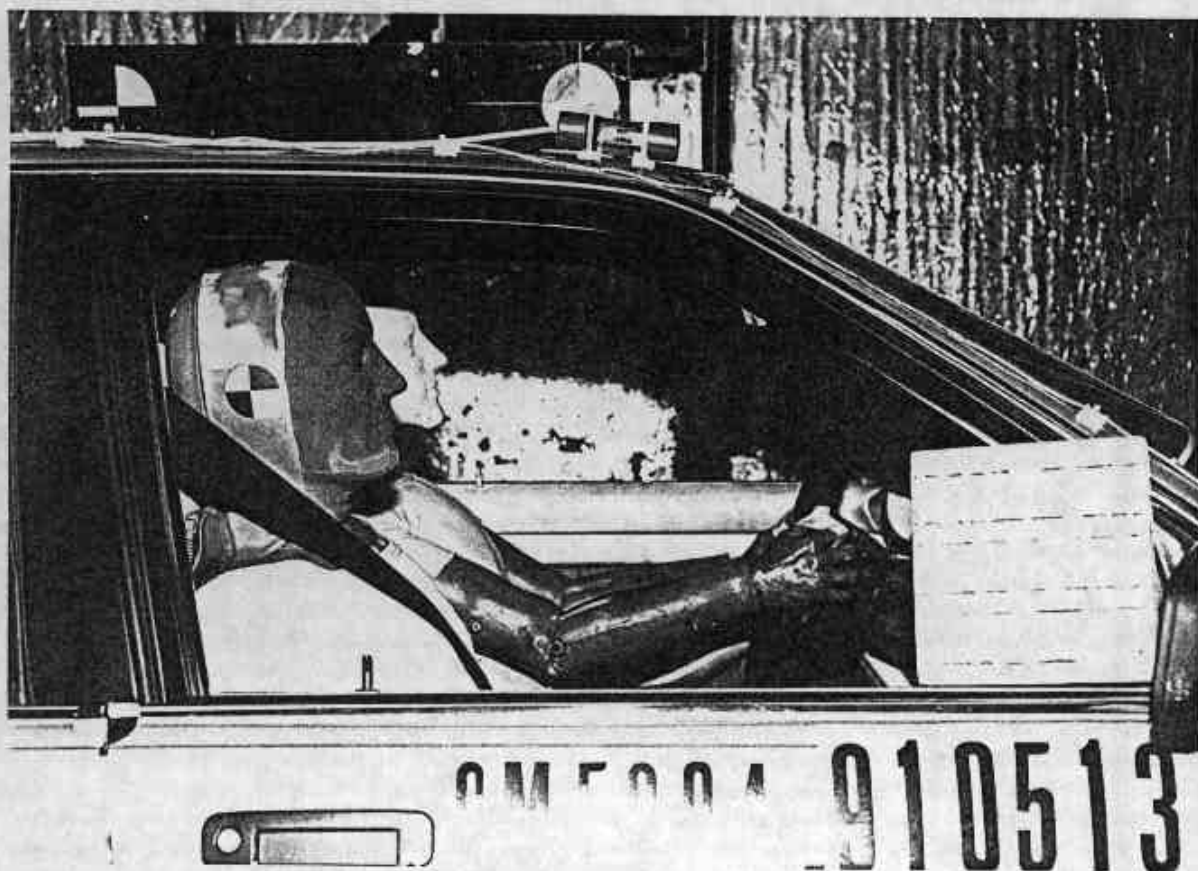
Figure A-27. PRE-TEST PASSENGER DUMMY POSITION VIEW
