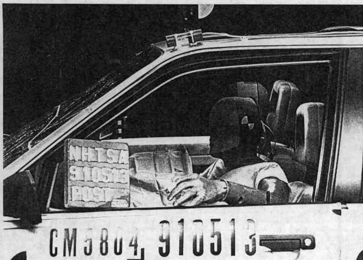
Figure A-26. POST-TEST DRIVER DUMMY POSITION VIEW
