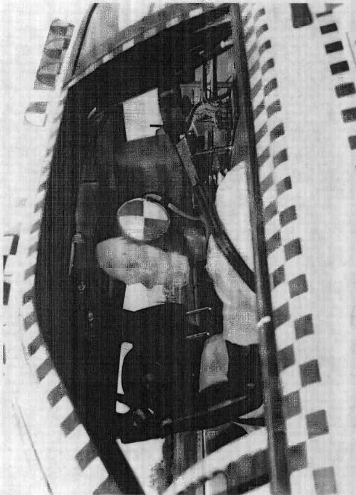
FIGURE A-27 POST-TEST DRIVER DUMMY POSITION
