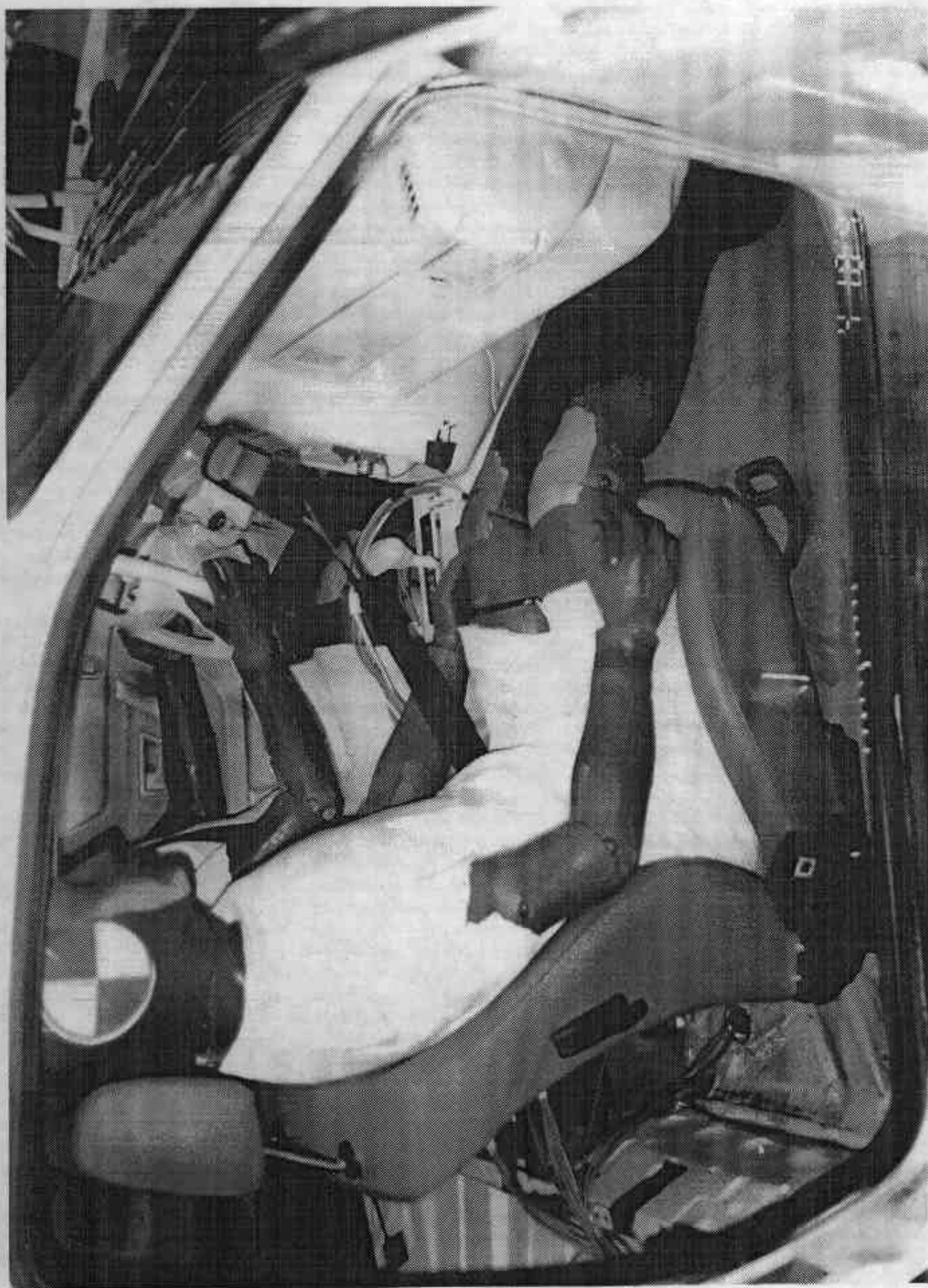
Figure A-32 PRE-TEST PASSENGER DUMMY AND INTERIOR VIEW
