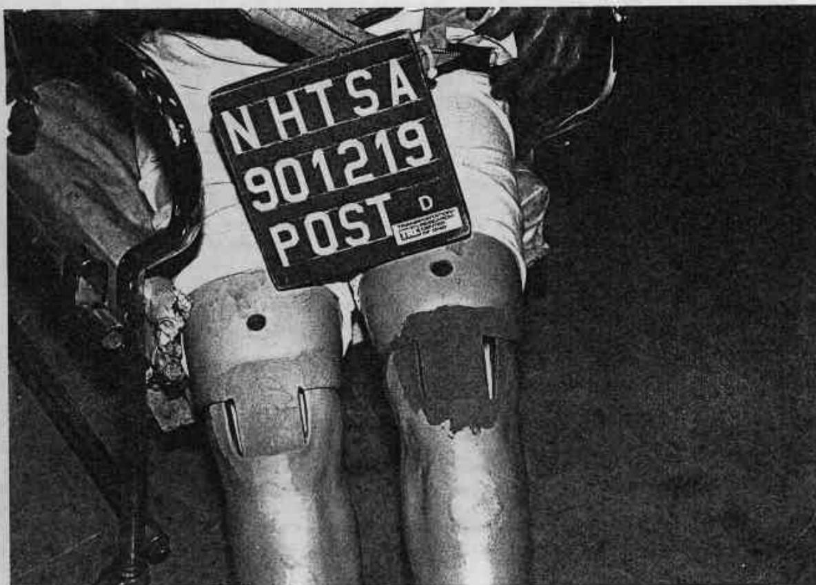
Figure A-38. POST-TEST DRIVER DUMMY KNEE CONTACT - VIEW 1
