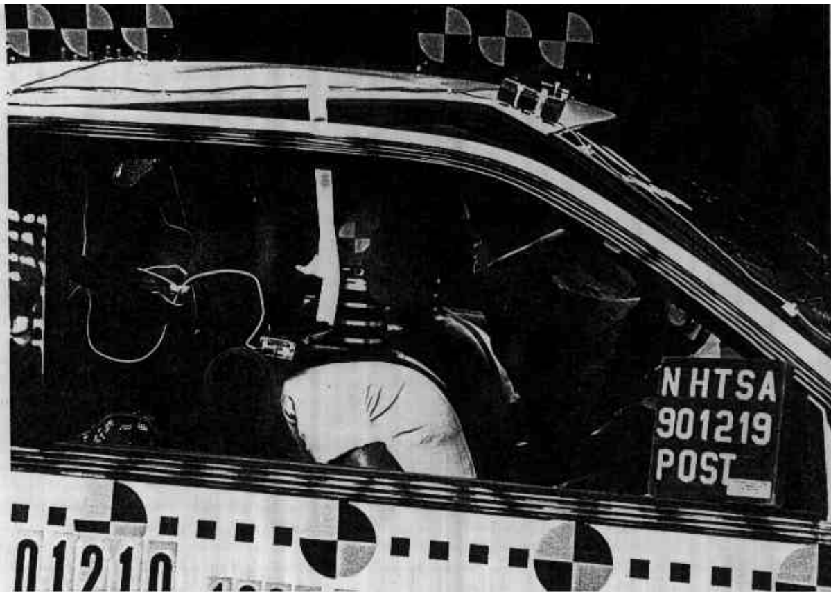
Figure A-27. POST-TEST PASSENGER DUMMY POSITION
