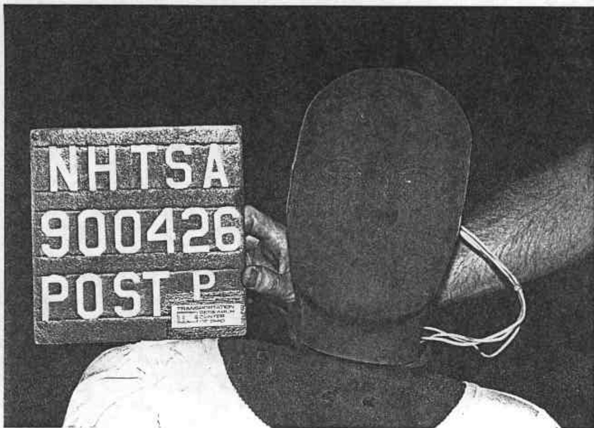
Figure A-37. POST-TEST PASSENGER DUMMY HEAD CONTACT VIEW
