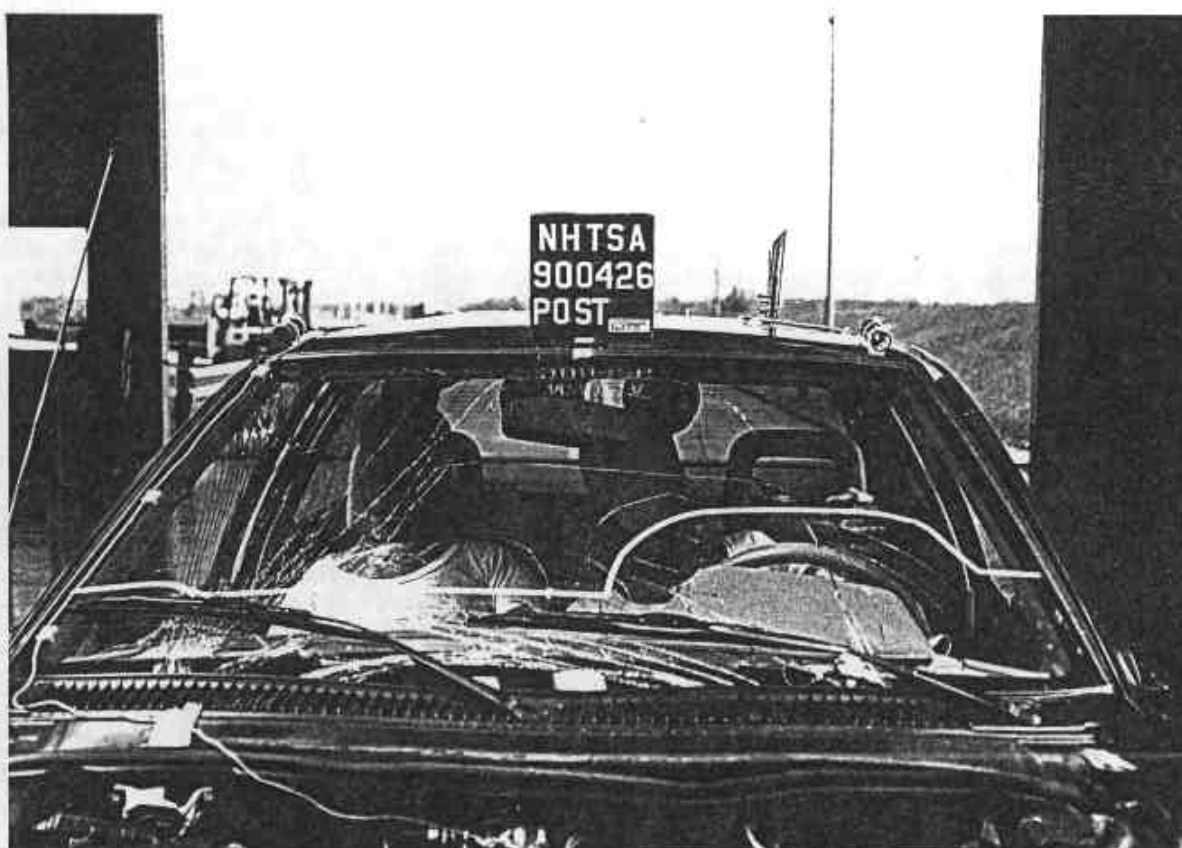
Figure A-14. POST-TEST WINDSHIELD VIEW
