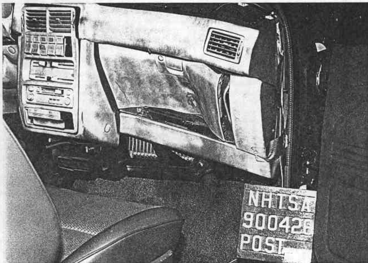
Figure A-39. POST-TEST PASSENGER DUMMY KNEE CONTACT - VIEW 2
