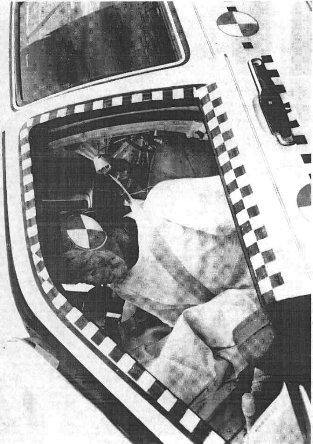
Figure A-29 POST-TEST DRIVER POSITION VIEW
