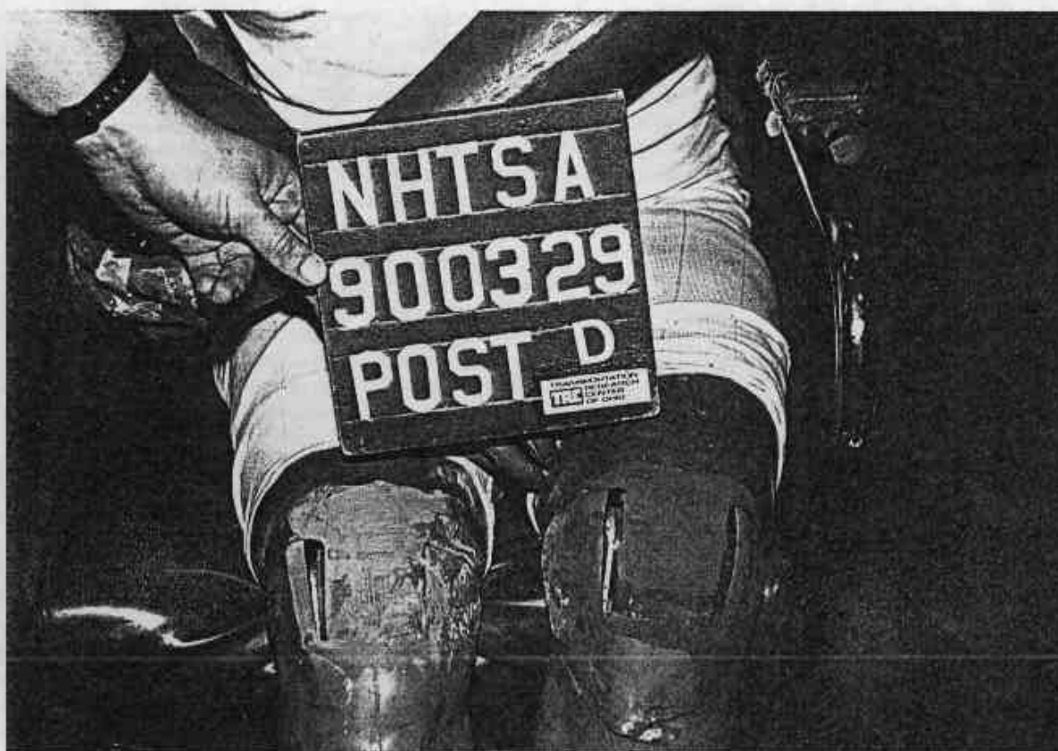
Figure A-36. POST-TEST DRIVER DUMMY KNEE CONTACT - VIEW 1
