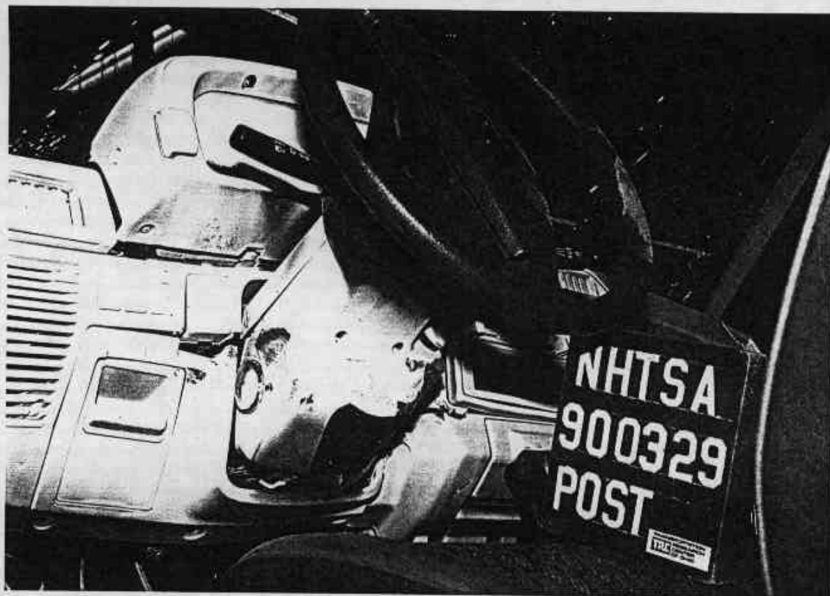
Figure A-37. POST-TEST DRIVER DUMMY KNEE CONTACT - VIEW 2
