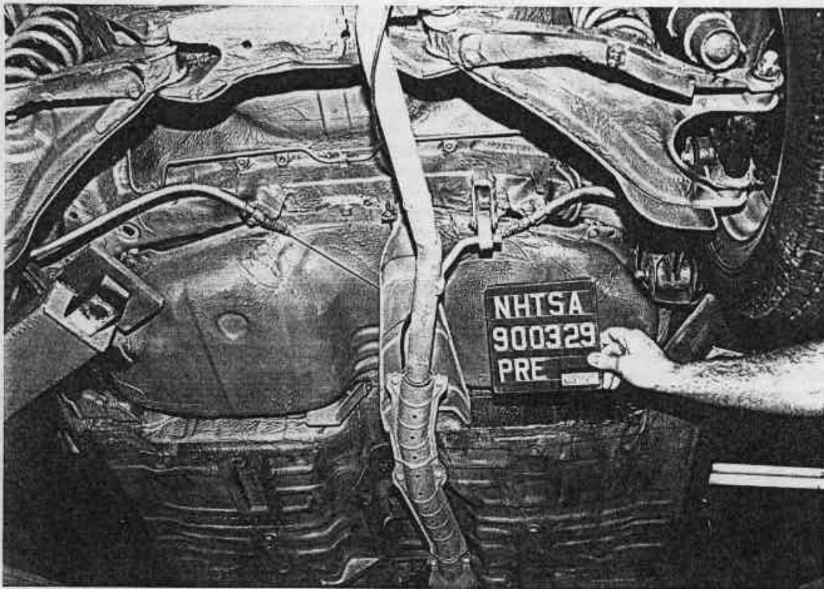
Figure A-23. PRE-TEST FUEL TANK VIEW
