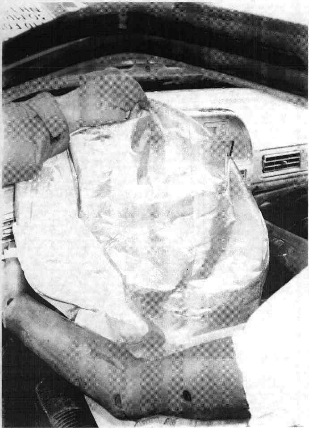
FIGURE A-34 POST-TEST DRIVER AIRBAG VIEW
