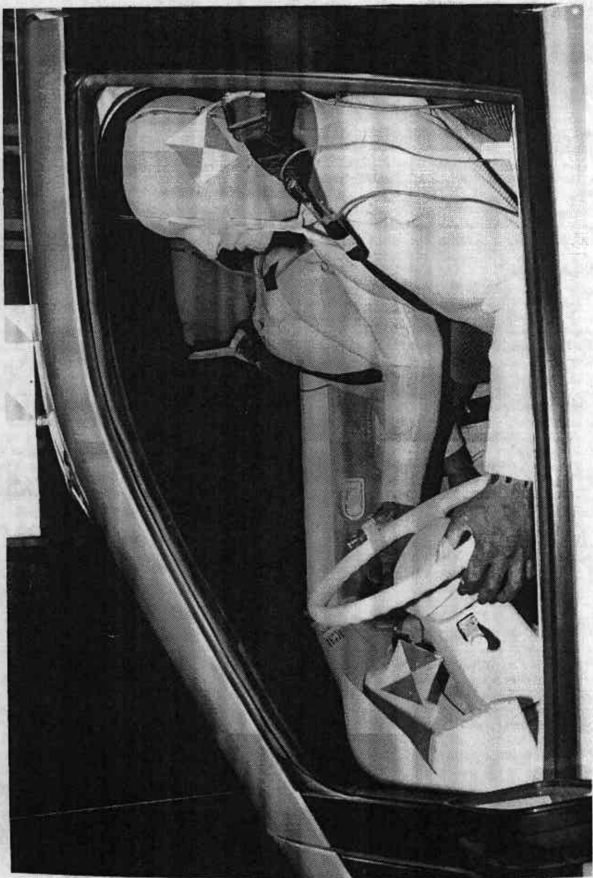
PRETEST DRIVER DUMMY POSITION VIEW
