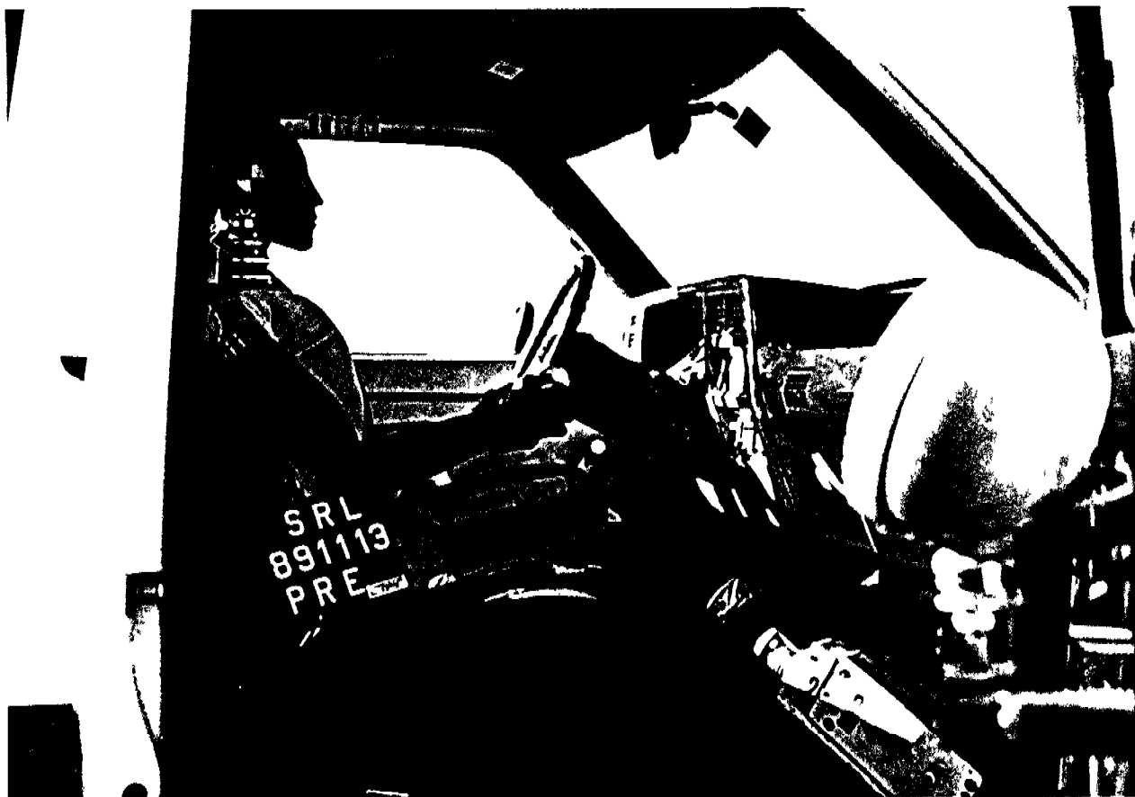
Figure A-6 PRE-TEST DRIVER DUMMY - VIEW 2
