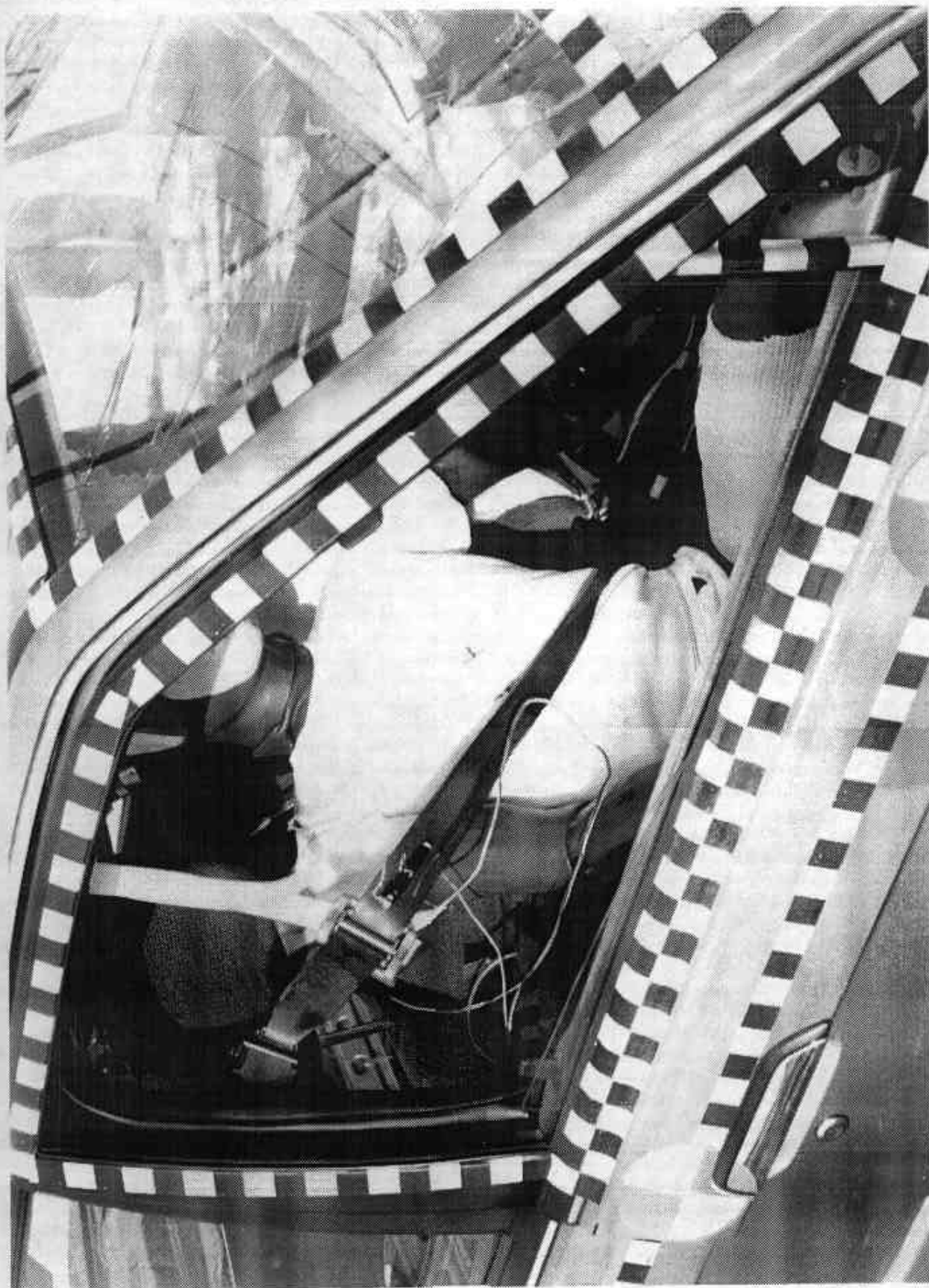
FIGURE A-25 POST-TEST PASSENGER POSITION VIEW
