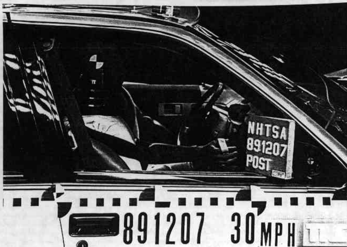
Figure A-27. POST-TEST PASSENGER DUMMY POSITION VIEW
