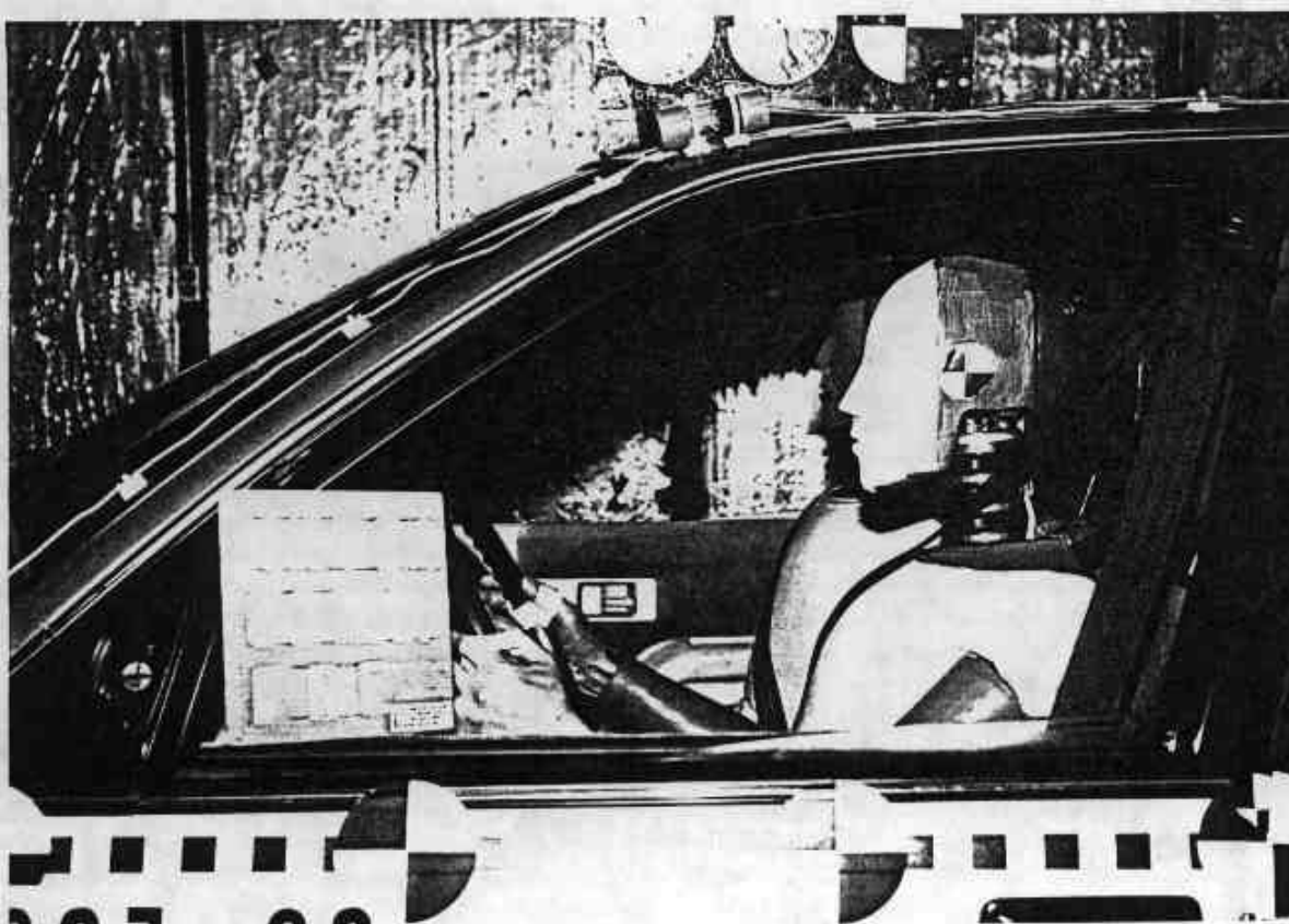
Figure A-24. PRE-TEST DRIVER DUMMY POSITION VIEW
