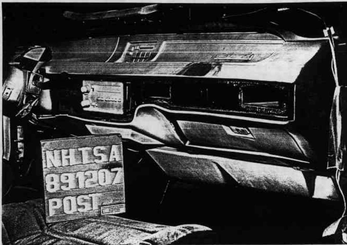
Figure A-39. POST-TEST RIGHT FRONT PASSENGER HEAD AND KNEE CONTACT VIEW
