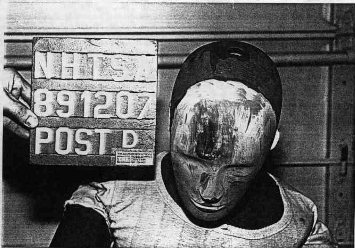
Figure A-34. POST-TEST DRIVER HEAD CONTACT - VIEW 1
