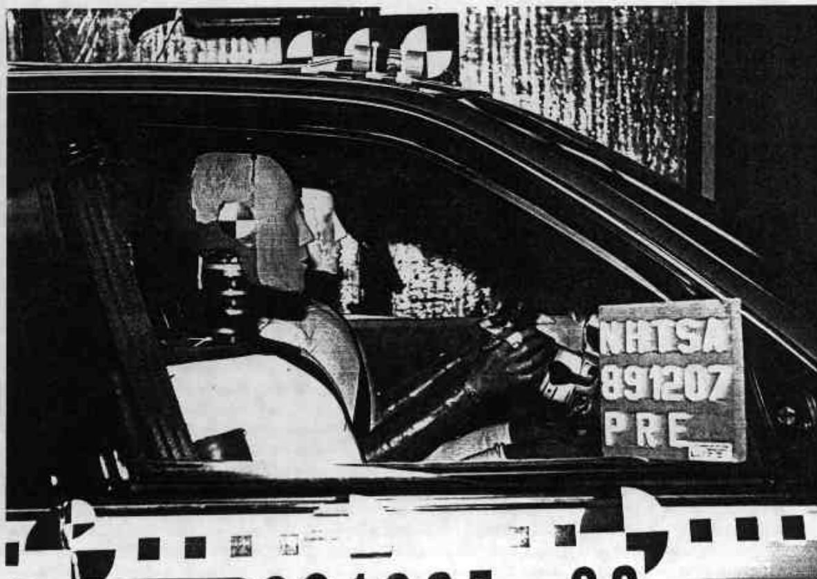
Figure A-26. PRE-TEST PASSENGER DUMMY POSITION VIEW
