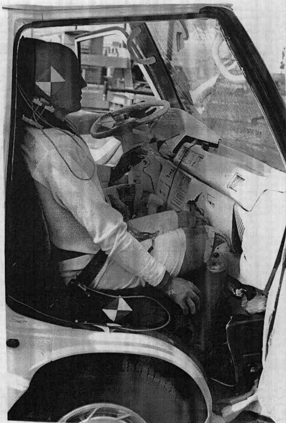
POSTTEST PASSENGER DUMMY (ATD) & VEHICLE INTERIOR VIEW (Door Open)
