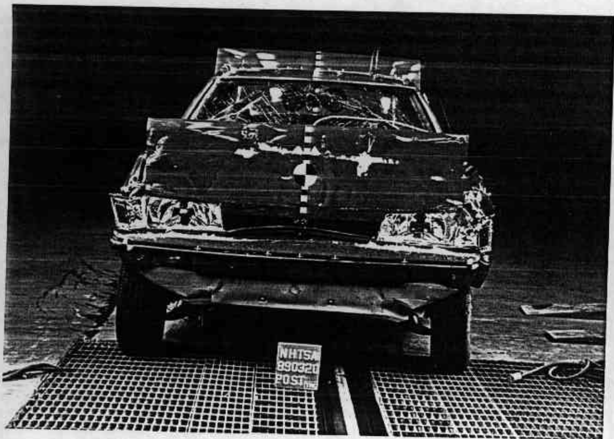
Figure A-2. POST-TEST FRONT VIEW A-2
