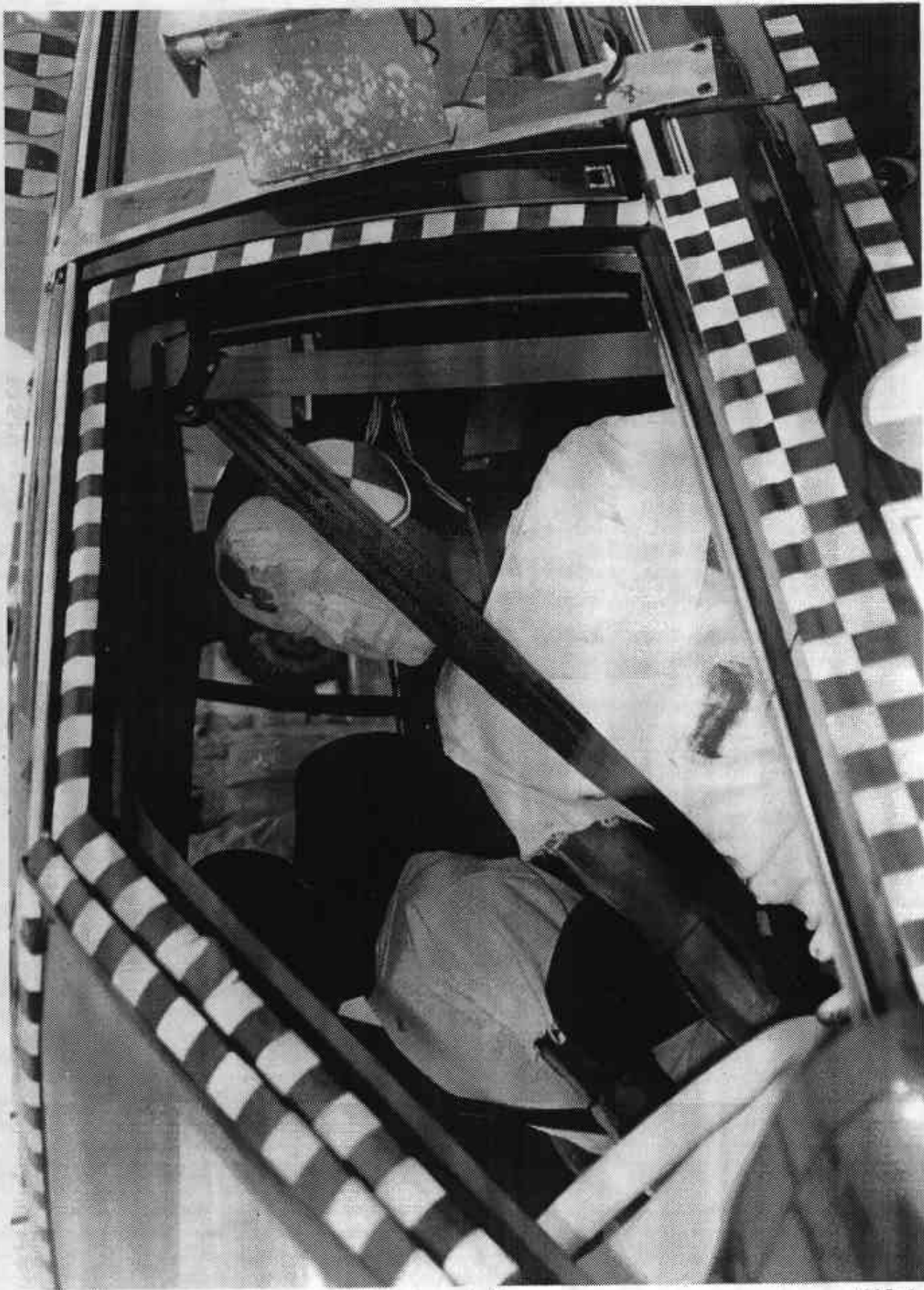
Figure A-26 POST-TEST DRIVER DUMMY POSITION
