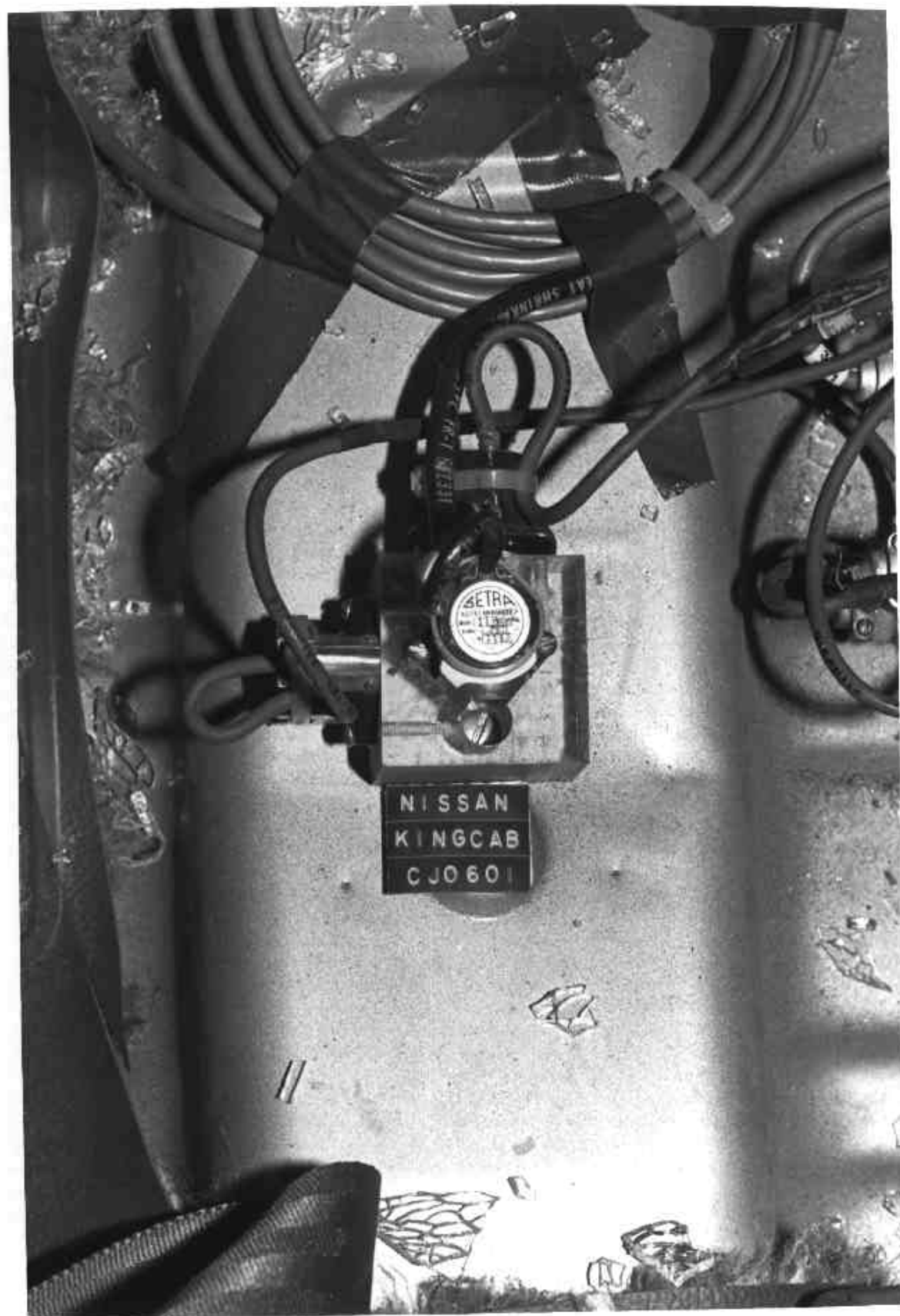
FIGURE 2-6 TRIAXIAL ACCELEROMETER MOUNTED AT VEHICLE C.G.
