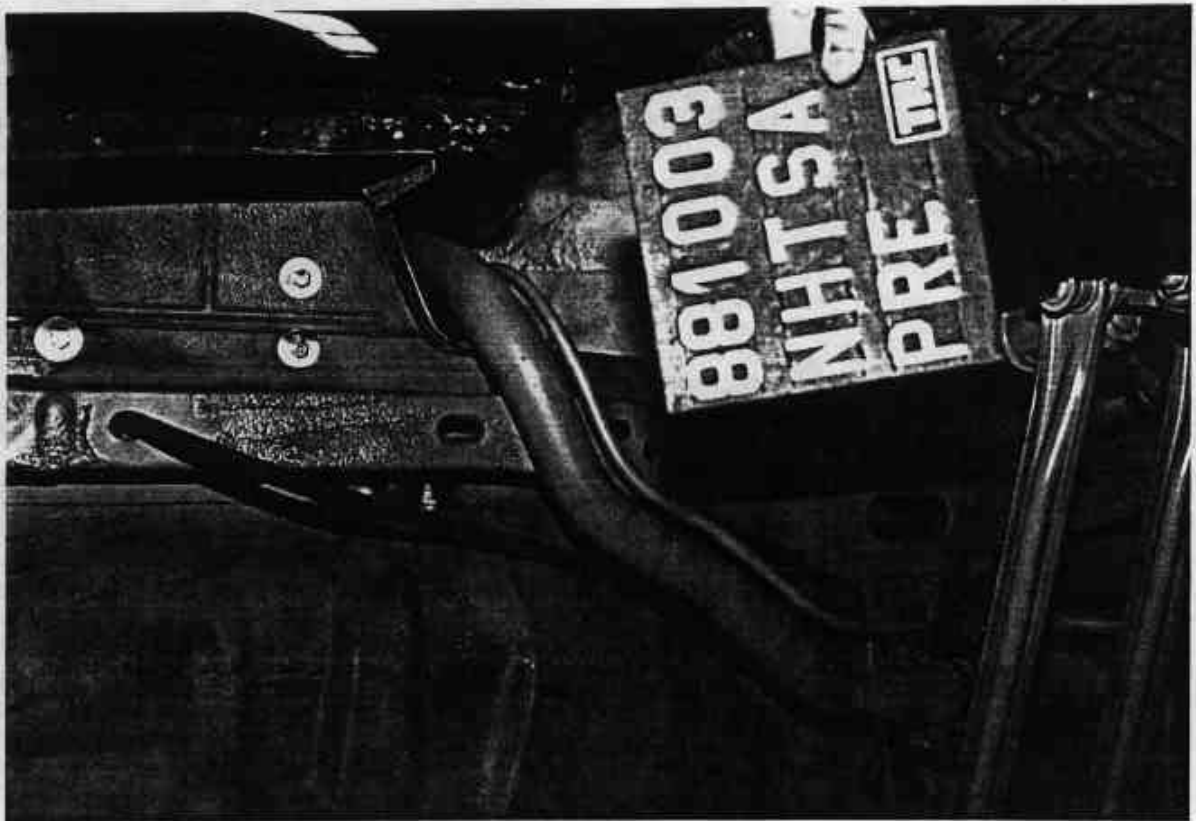
Figure A-24. PRE-TEST FUEL FILLER NECK VIEW A-14
