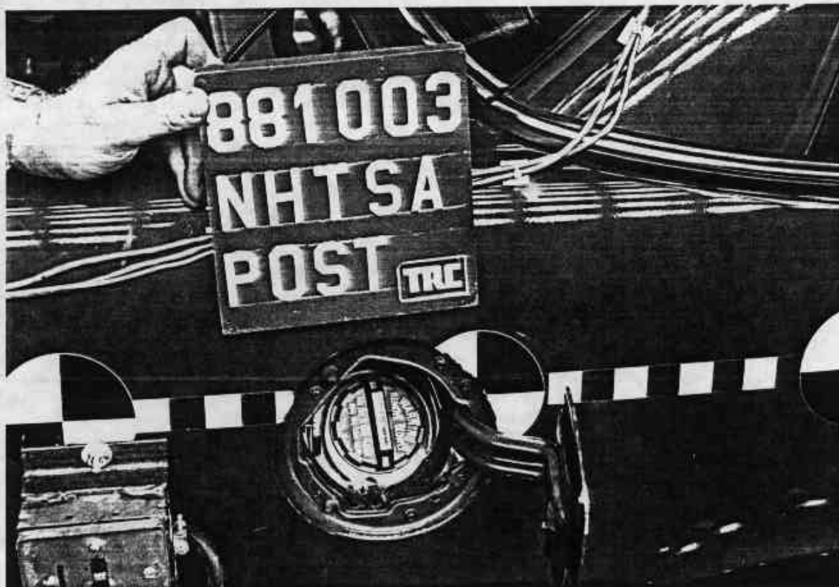
Figure A-17. POST-TEST FUEL FILLER CAP VIEW
