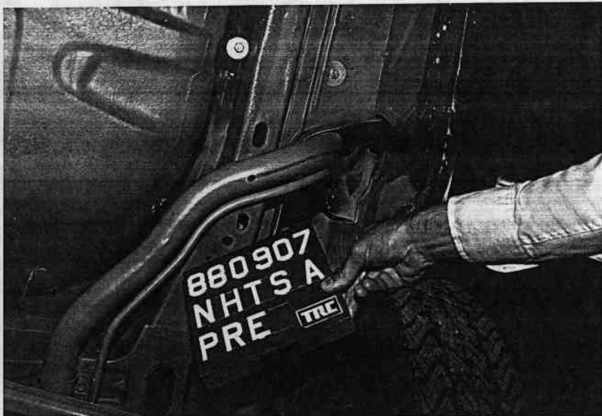
Figure A-25. PRE-TEST FUEL FILLER NECK VIEW
