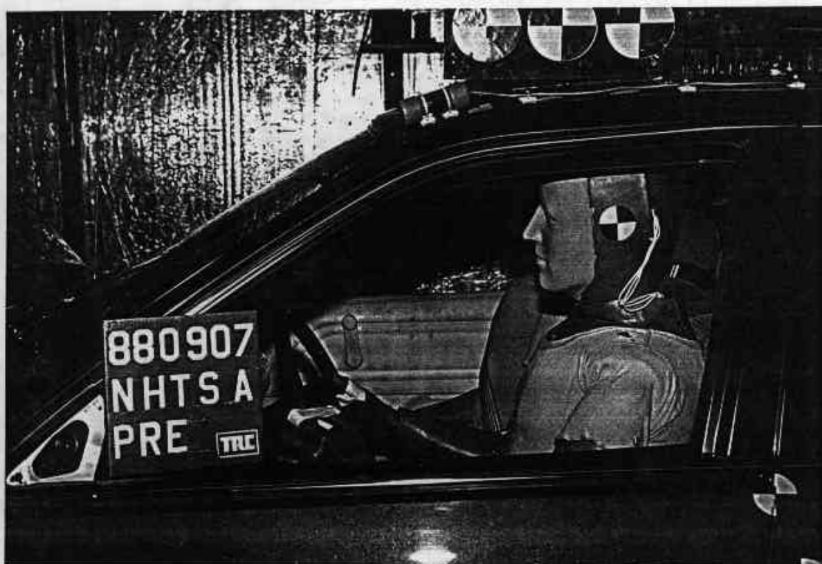
Figure A-26. PRE-TEST DRIVER DUMMY POSITION VIEW A-15
