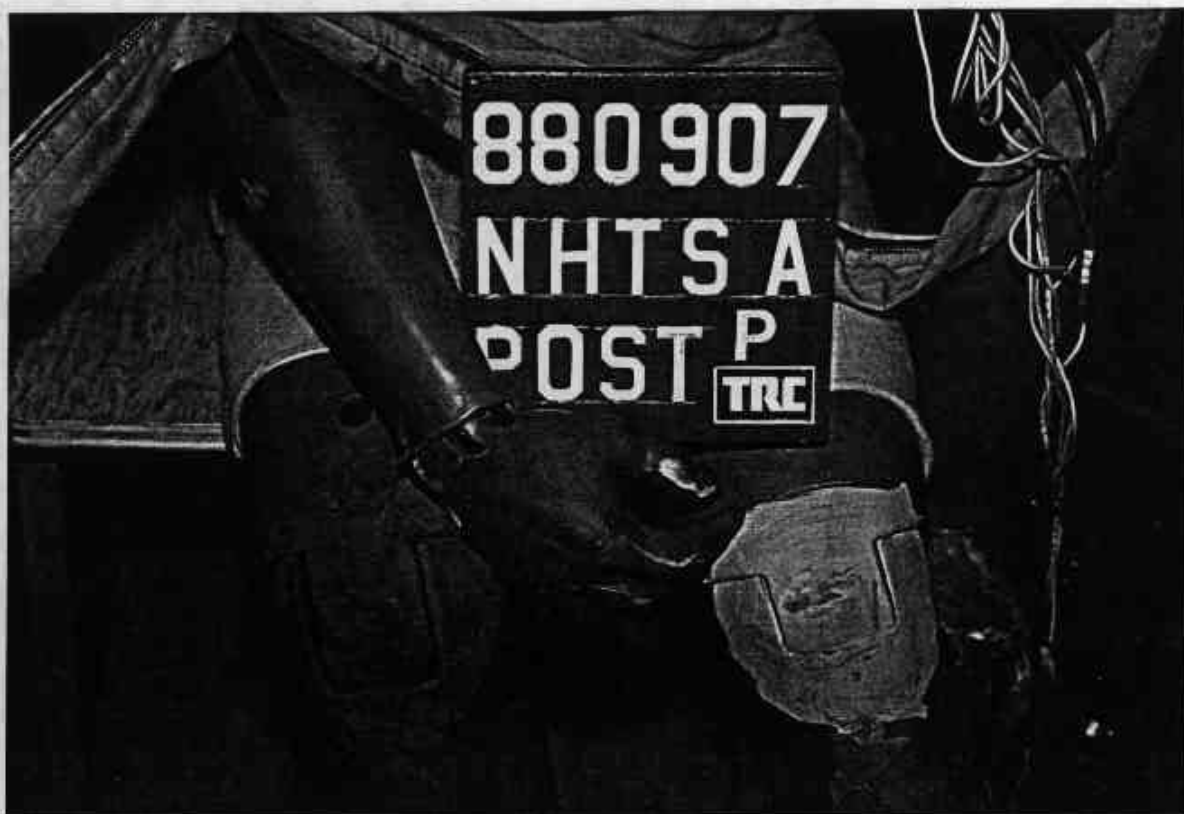
Figure A-44. POST-TEST PASSENGER DUMMY HEAD/KNEE CONTACT - VIEW 1
