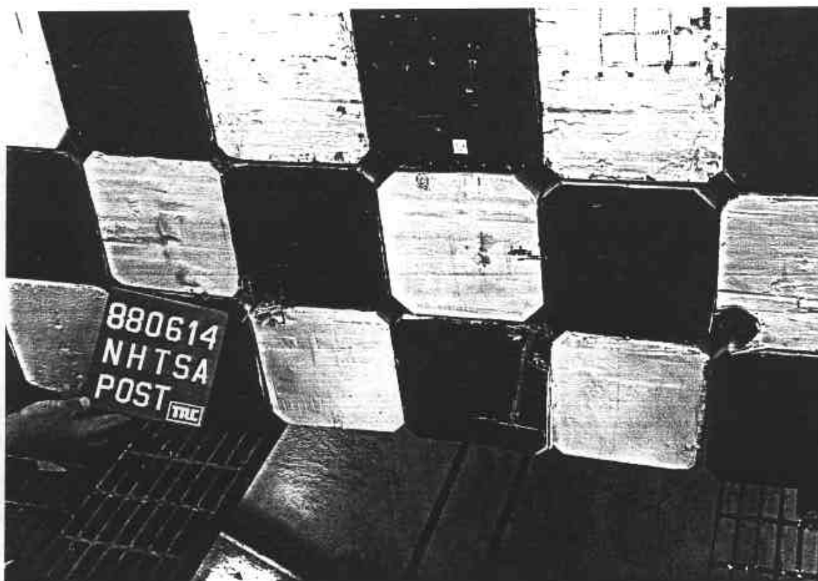
Figure A-40. POST-TEST LOAD CELL BARRIER DAMAGE - VIEW 1
