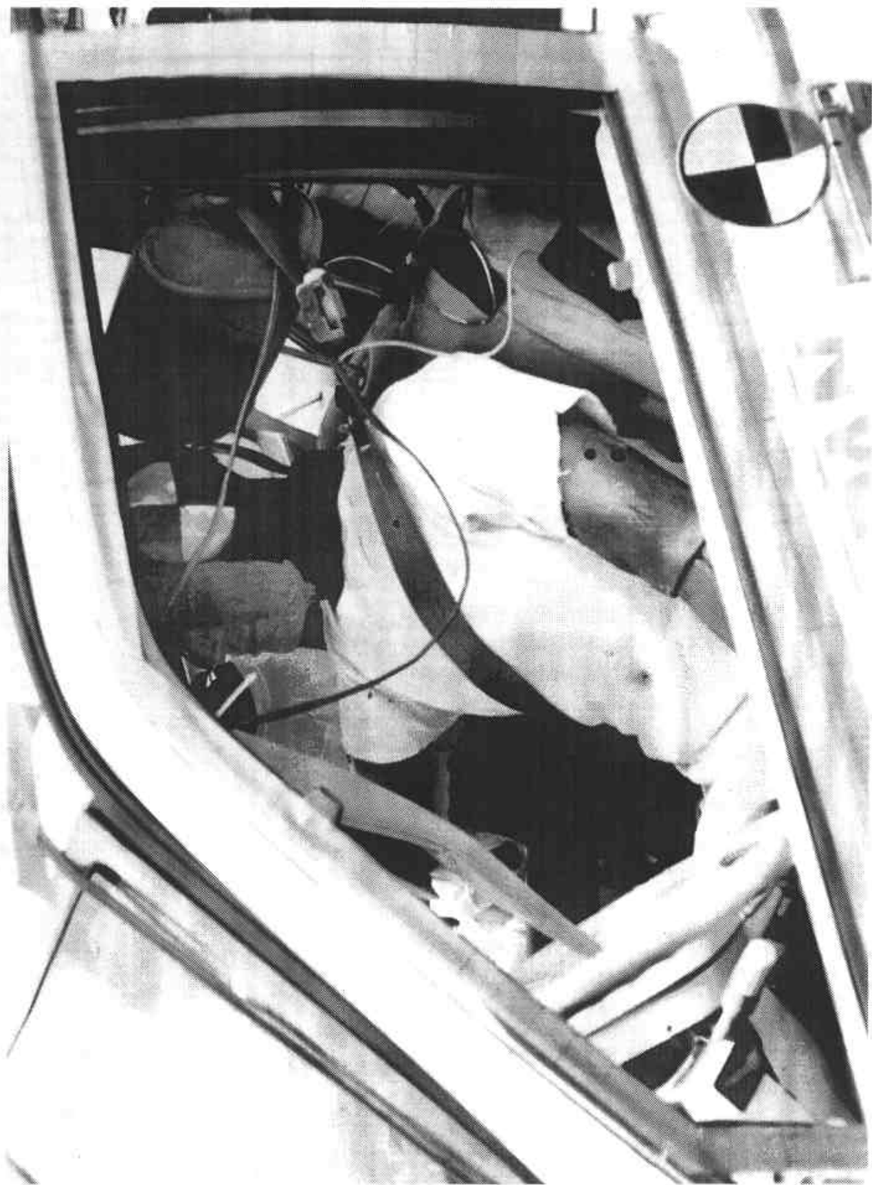
Figure A-22 POST-TEST DRIVER POSITION VIEW
