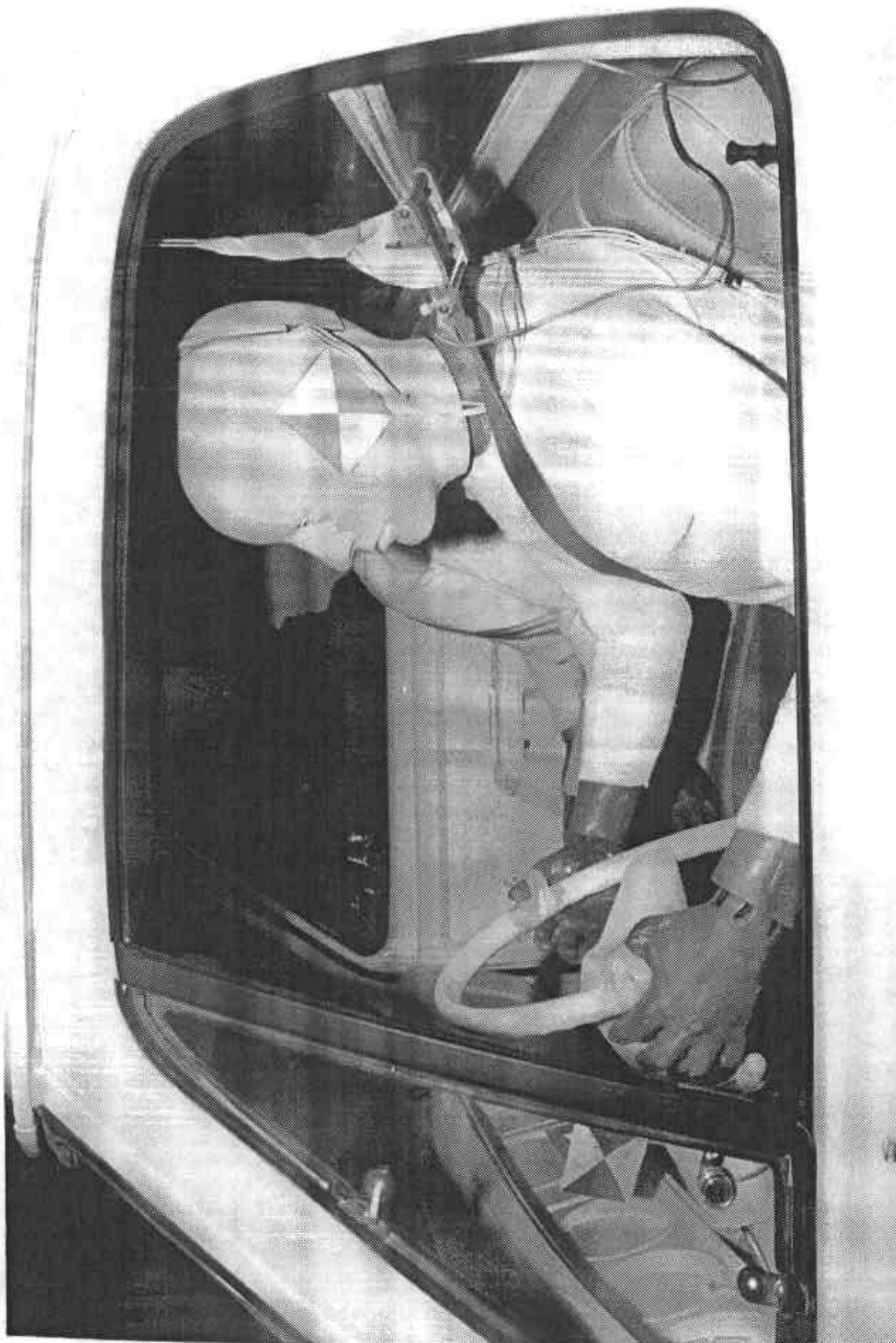
PRETEST DRIVER DUMMY (ATD) POSITION VIEW
