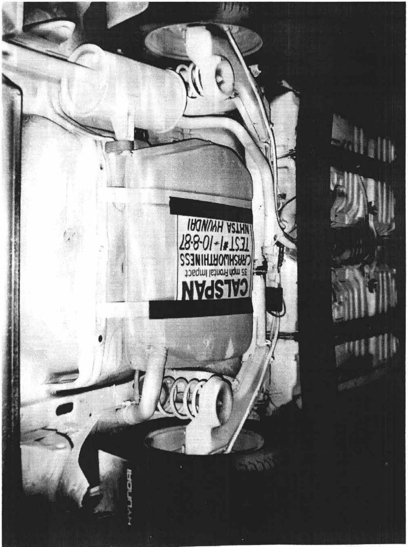
Figure A-15 PRE-TEST REAR VIEW UNDERBODY
