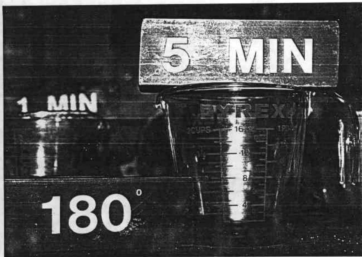
Figure 44. POST-TEST STODDARD LEAKAGE - VIEW 3 A-23
