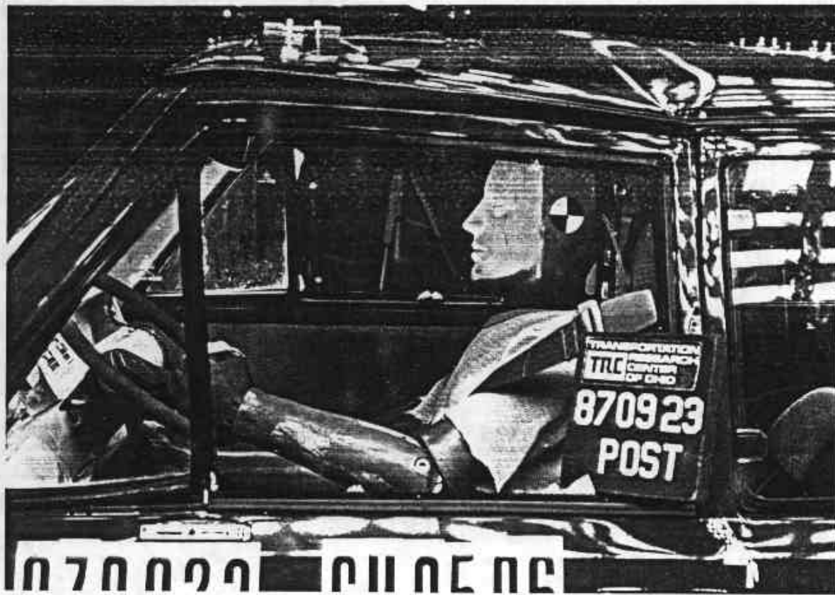
Figure 25. POST-TEST DRIVER DUMMY POSITION VIEW
