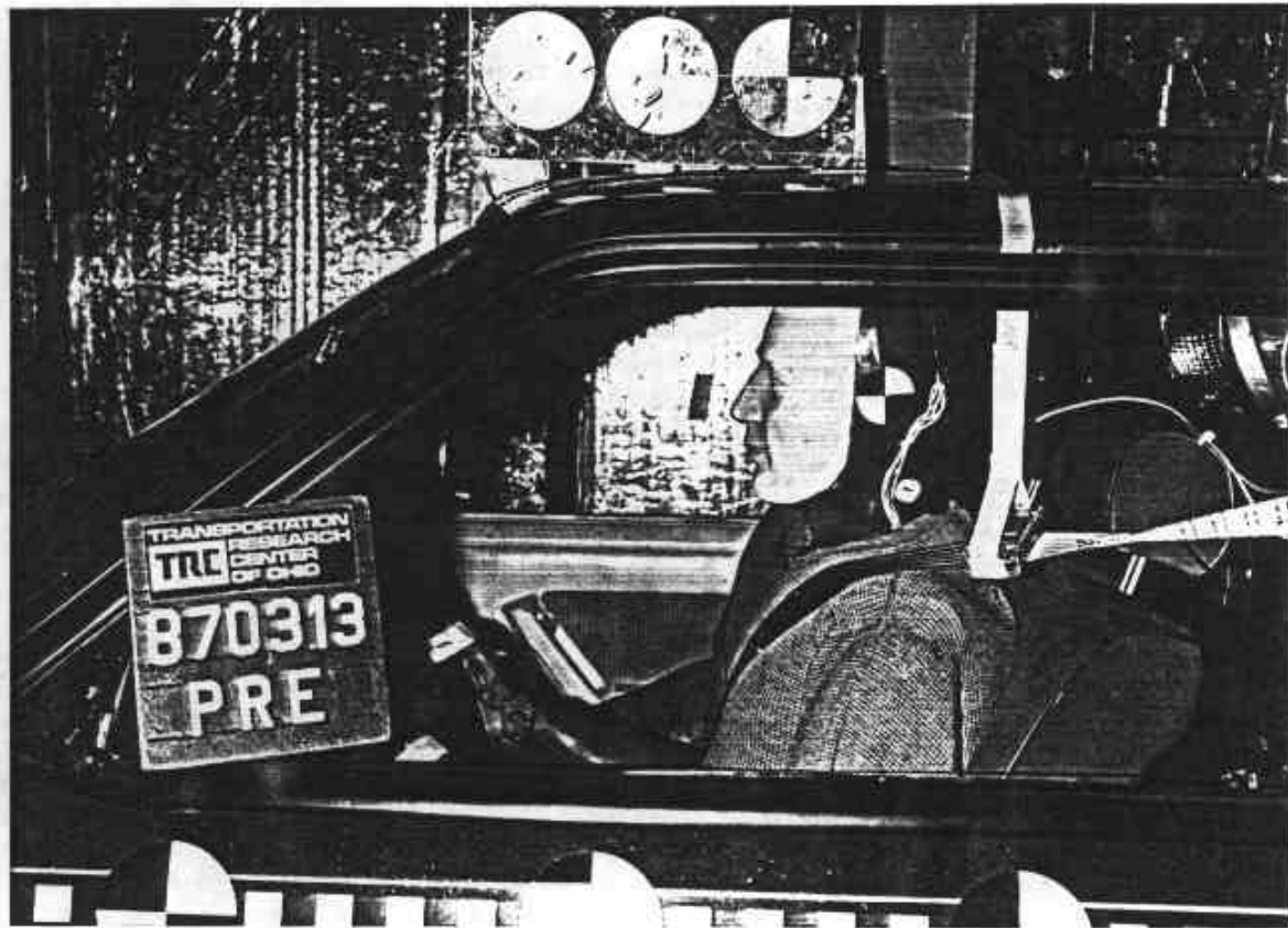
Figure 20. PRE-TEST DRIVER DUMMY POSITION VIEW
