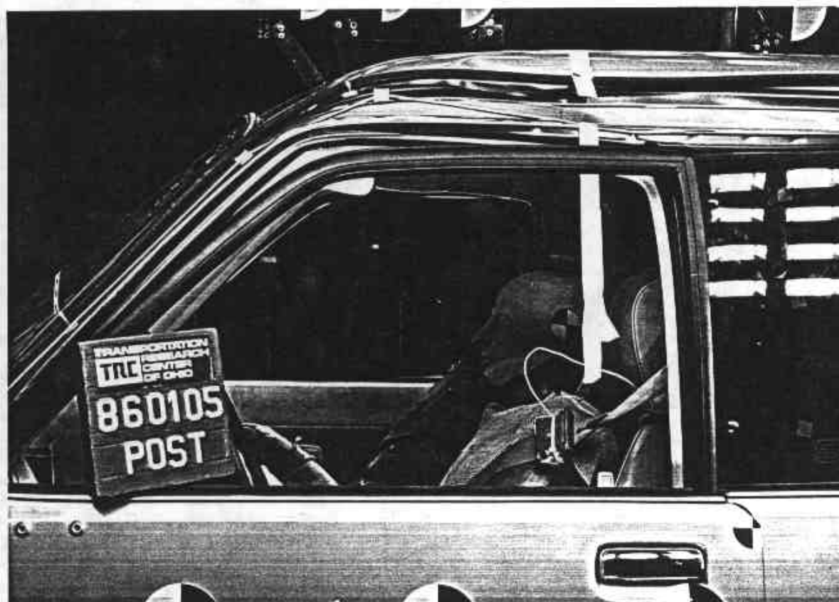
Figure 22. POST-TEST DRIVER DUMMY POSITION VIEW
