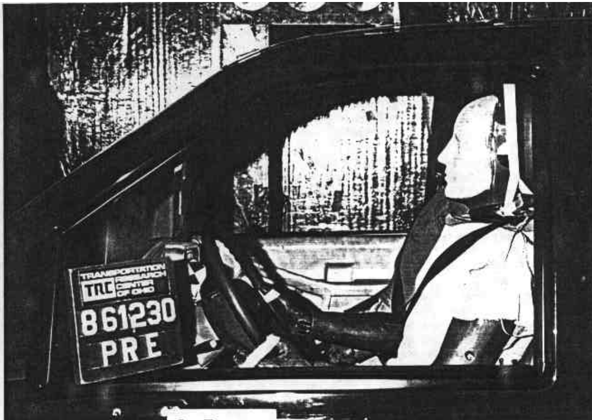
Figure 21. PRE-TEST DRIVER DUMMY POSITION VIEW
