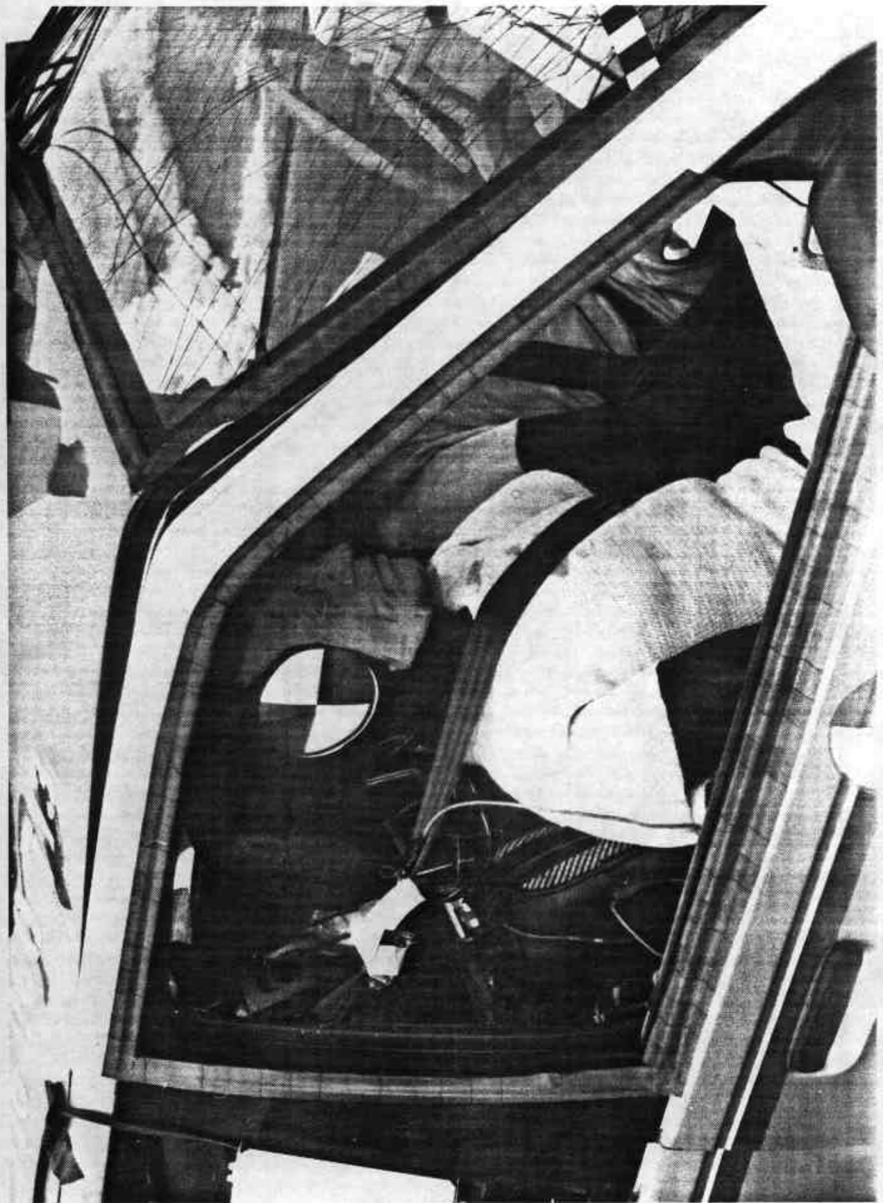
Figure A-26 POST-TEST PASSENGER POSITION VIEW
