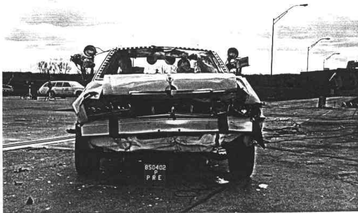
Figure A-34. POST-TEST PARTNER VEHICLE FRONT VIEW A-18
