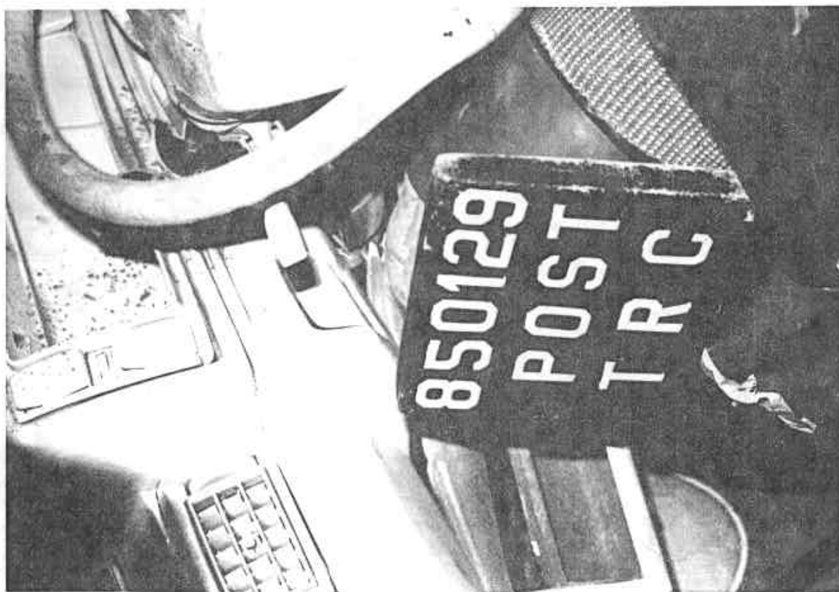
Figure 22. POST-TEST DRIVER DUMMY HEAD CONTACT AREA
