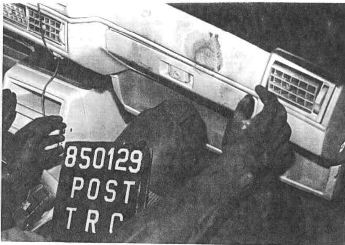
Figure 23. POST-TEST PASSENGER DUMMY HEAD/KNEE CONTACT
