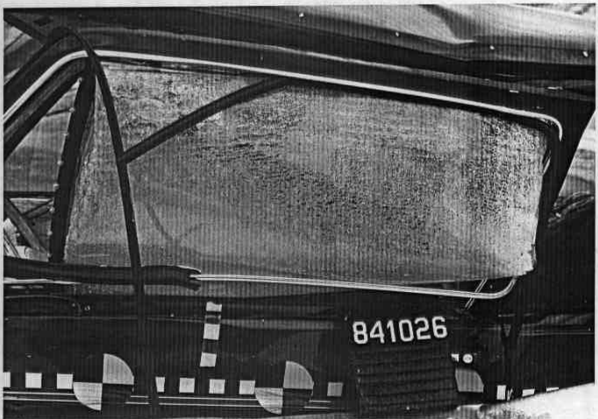
Figure A-24. POST-TEST MODIFIED WINDOW A-13
