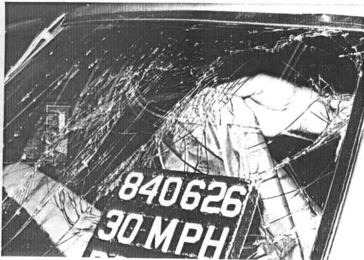
Figure B-24. WINDSHIELD DAMAGE B-13
