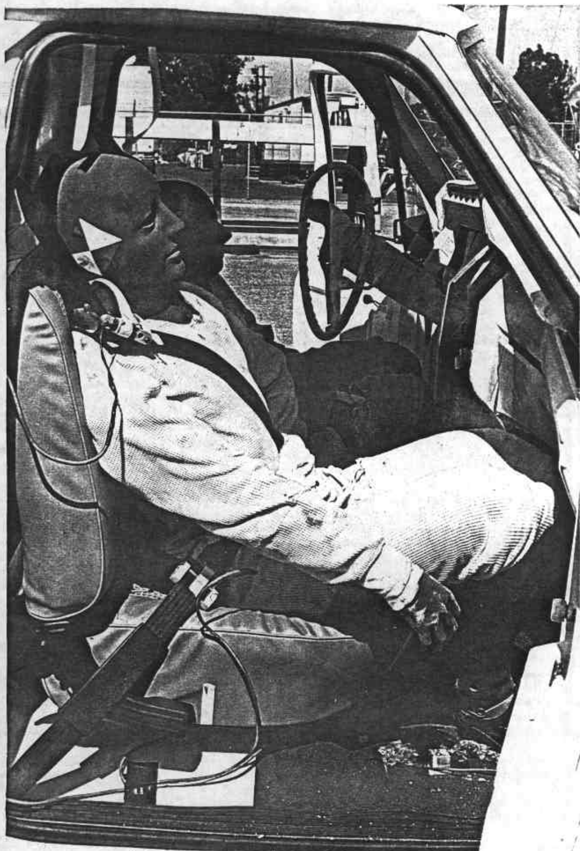
A-17 PASSENGER ATD GENERAL POSITION - POSTTEST
