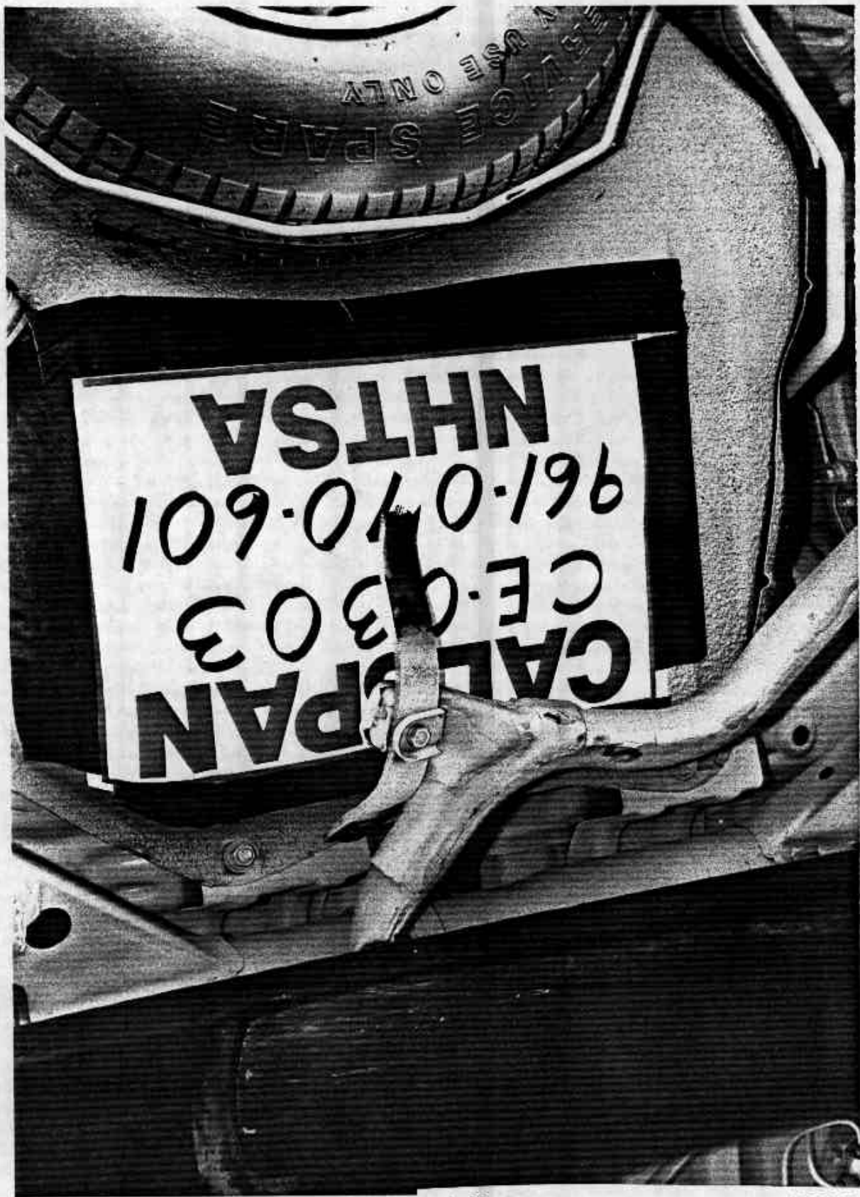
Figure A-21 POST-TEST FUEL TANK AND BROKEN EXHAUST SUPPORT STRAP
