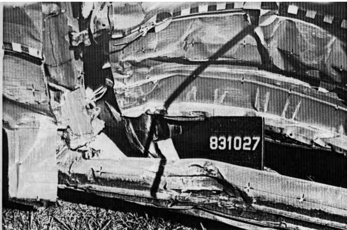
Figure A-25. POST-TEST VEHICLE DAMAGE - VIEW 3
