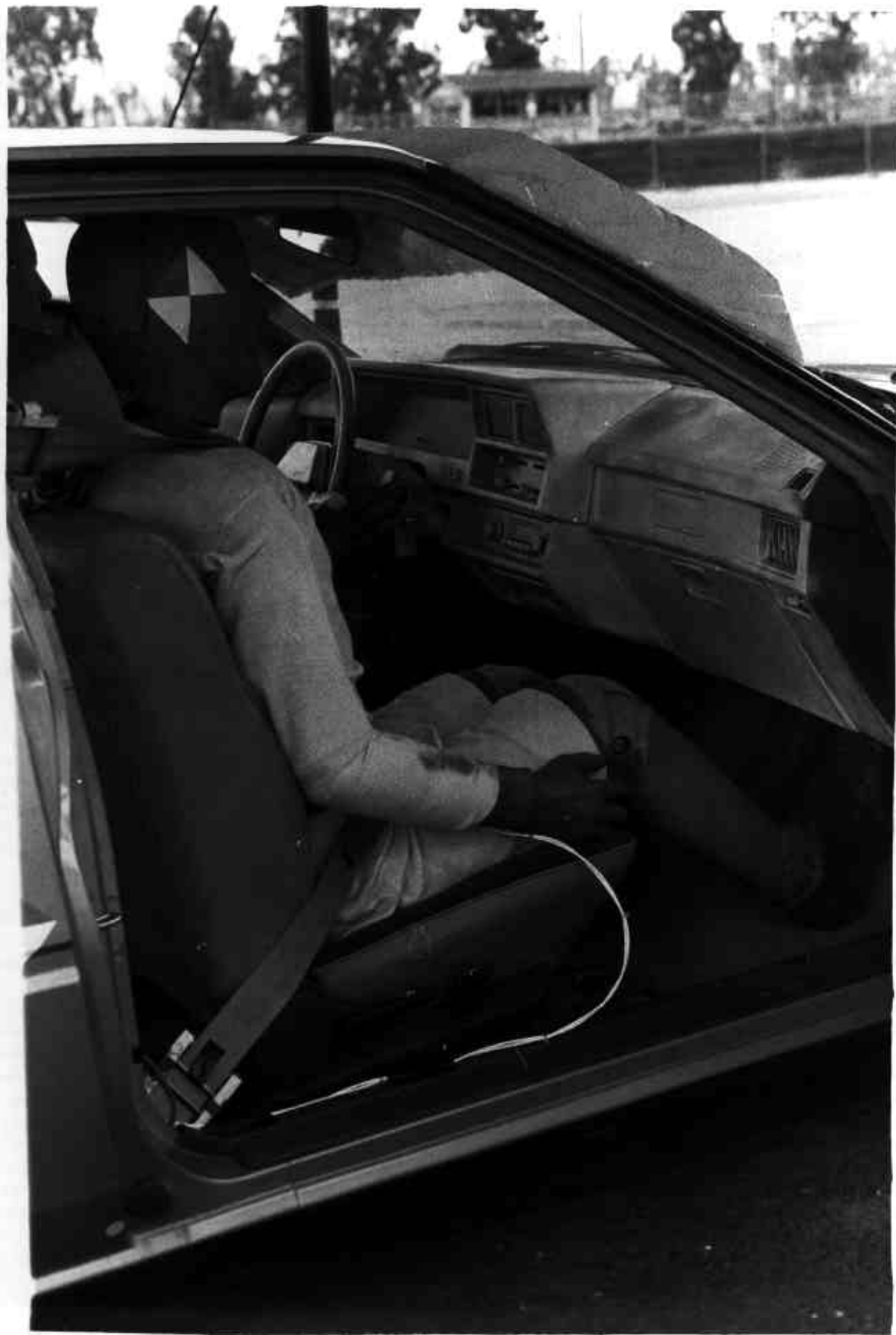
A-7 PASSENGER ATD GENERAL POSITION, PRETEST
