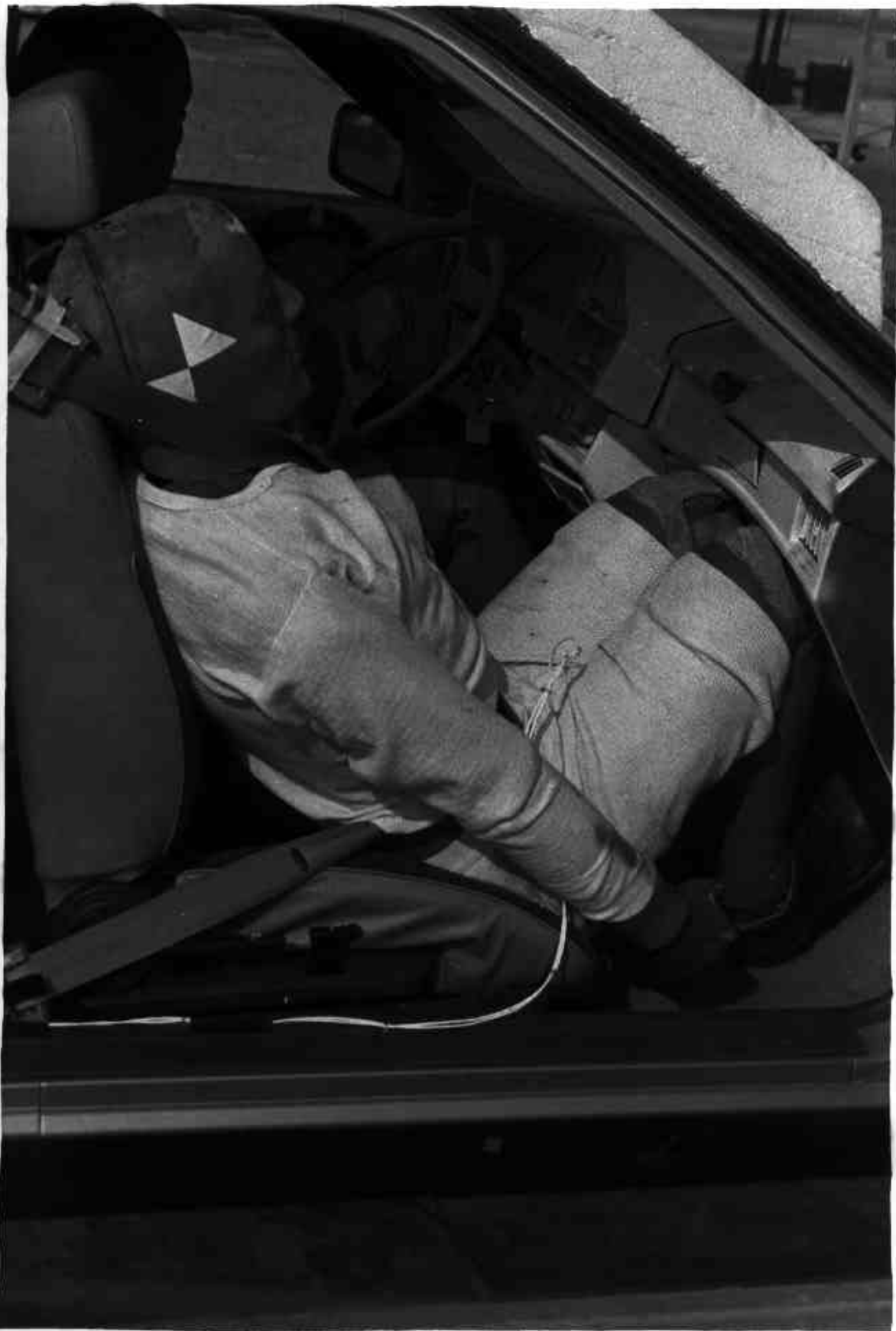
A-17 PASSENGER ATD GENERAL POSITION, POSTTEST
