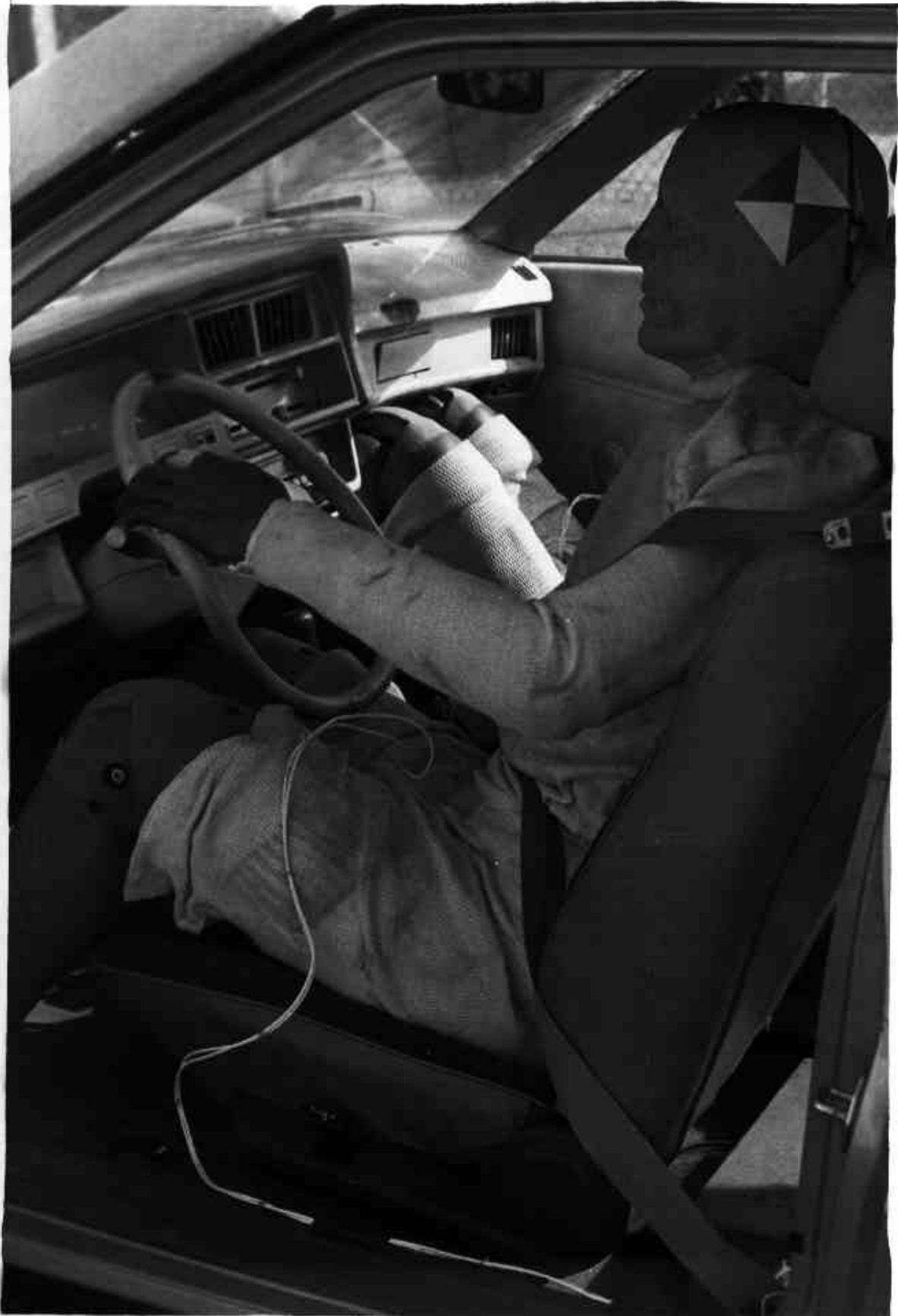
A-16 DRIVER ATD GENERAL POSITION, POSTTEST
