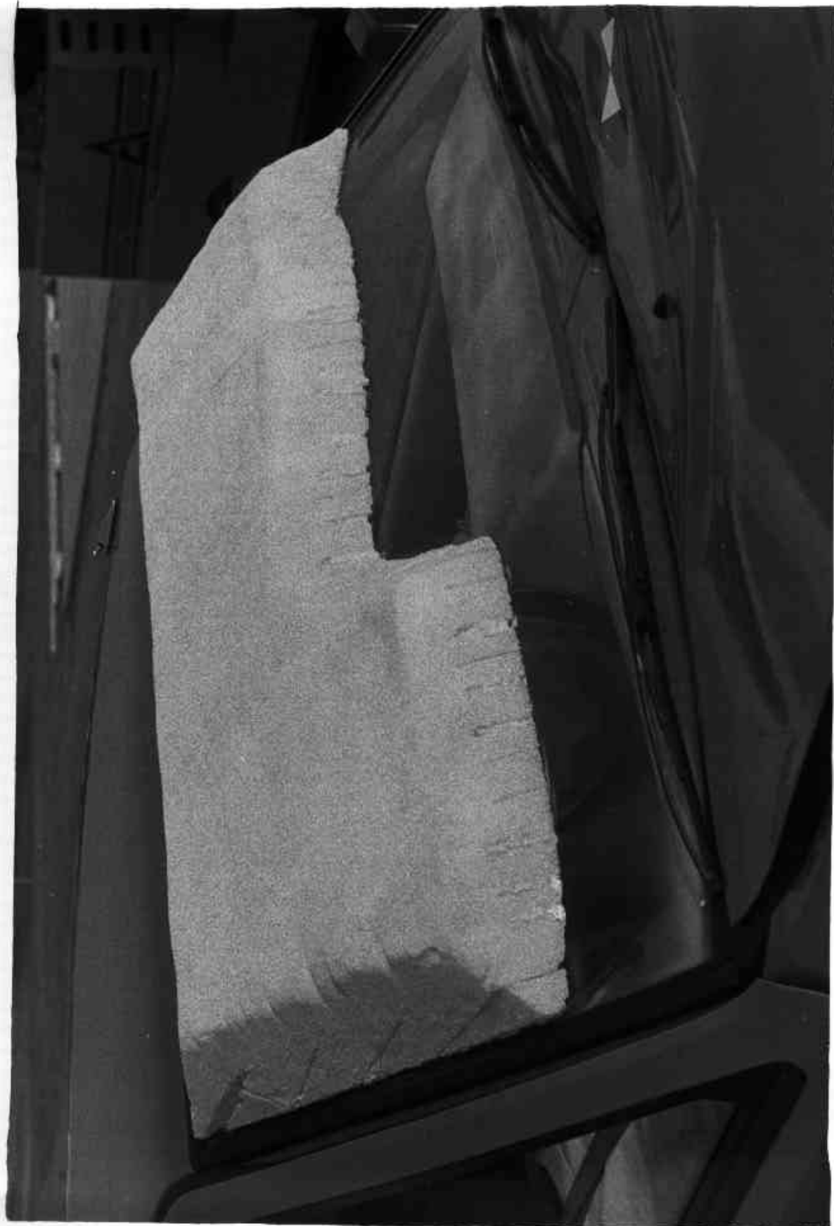
A-13 WINDSHIELD WITH STYROFOAM, POSTTEST
