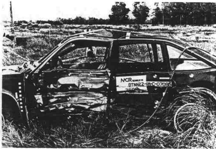
FIGURE 13. CLOSE UP OF VEHICLE DAMAGE - DRIVERS SIDE
