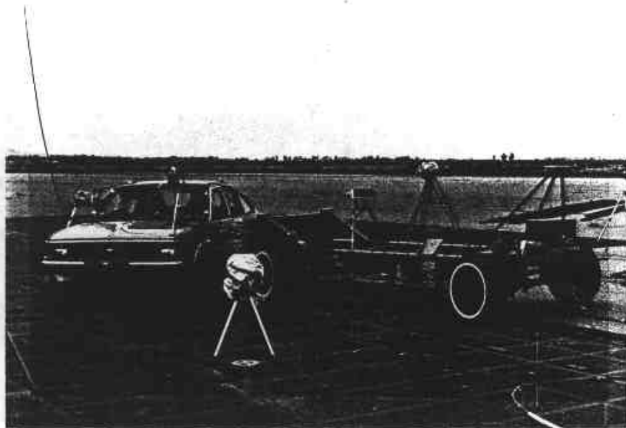
FIGURE 1. CRASH CONFIGURATION - DRIVERS SIDE FRONT
