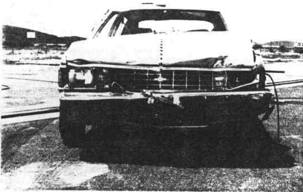
FIGURE A-2. POST-TEST FRONT VIEW OF "BULLET" VEHICLE - 90° TWO VEHICLE MOVING SIDE IMPACT - 1981 CITATION AT 35 MPH TO 1982 VOLKSWAGEN RABBIT AT 17.5 MPH.
