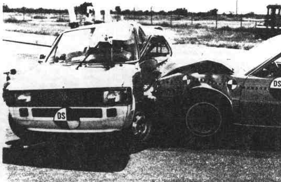
FIGURE A-12. POST-TEST FRONT VIEW OF VOLKSWAGEN RABBIT - 90° TWO VEHICLE MOVING SIDE IMPACT - 1981 CITATION AT 35 MPH TO 1982 VOLKSWAGEN RABBIT AT 17.5 MPH.
