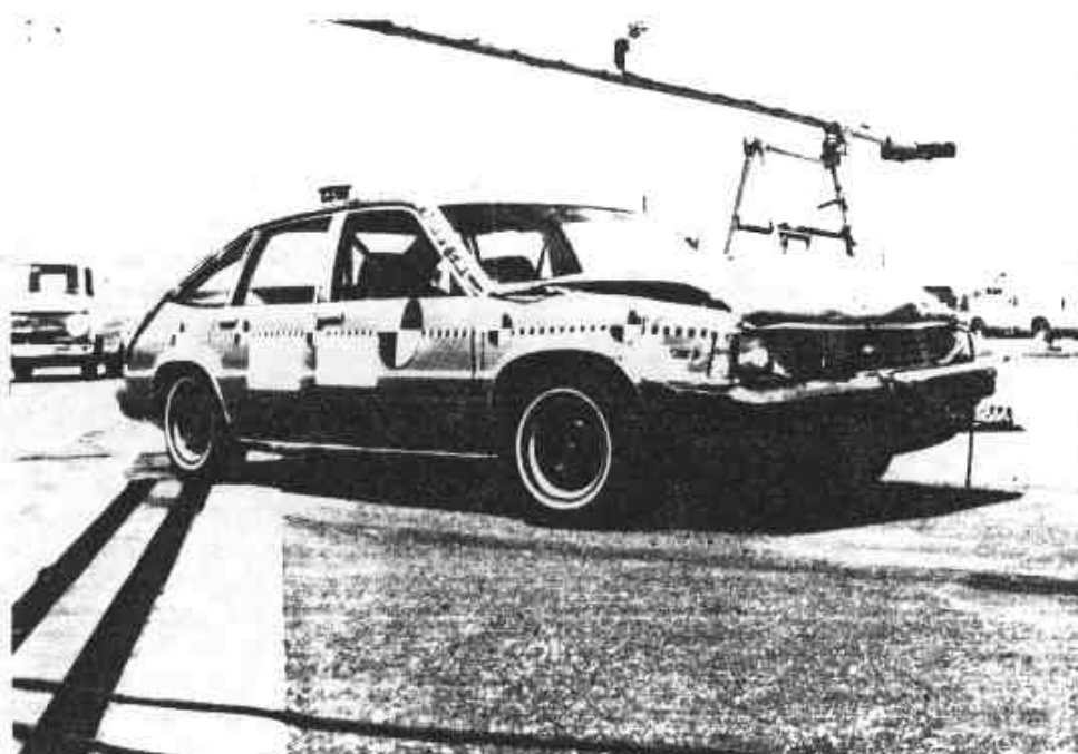
FIGURE A-6. POST-TEST RIGHT SIDE VIEW OF "BULLET" VEHICLE - 90° TWO VEHICLE MOVING SIDE IMPACT - 1981 CITATION AT 35 MPH TO 1982 VOLKSWAGEN RABBIT AT 17.5 MPH.
