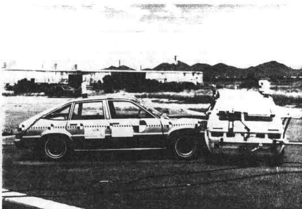
FIGURE A-20. POST-TEST REAR VIEW OF VOLKSWAGEN RABBIT - 90° TWO VEHICLE MOVING SIDE IMPACT - 1981 CITATION AT 35 MPH TO 1982 VOLKSWAGEN RABBIT AT 17.5 MPH.
