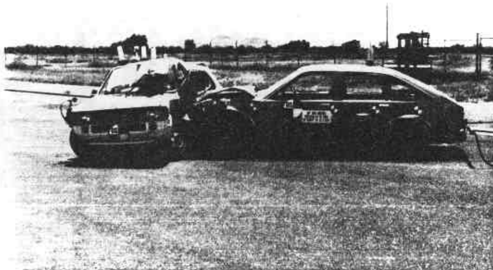
FIGURE A-8. POST-TEST FRONT VIEW OF VEHICLE MATCHUP - 90° TWO VEHICLE MOVING SIDE IMPACT - 1981 CITATION AT 35 MPH TO 1982 VOLKSWAGEN RABBIT AT 17.5 MPH.
