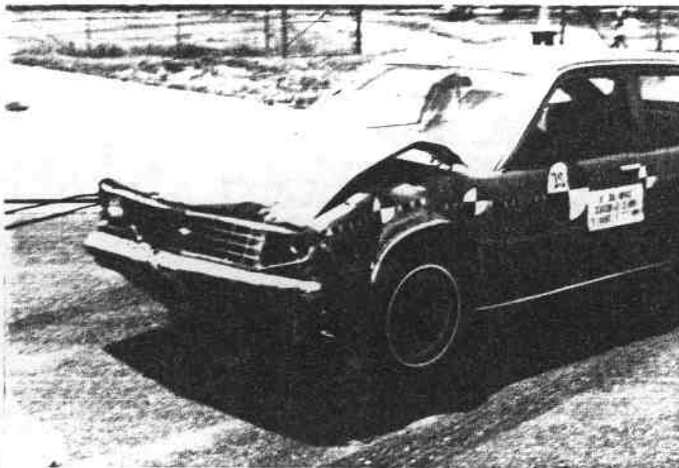
FIGURE A-4. POST-TEST LEFT SIDE VIEW OF "BULLET" VEHICLE - 90° TWO VEHICLE MOVING SIDE IMPACT - 1981 CITATION AT 35 MPH TO 1982 VOLKSWAGEN RABBIT AT 17.5 MPH.
